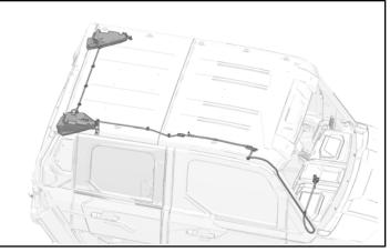
1. Install rear audio harness ④ along roof with two edge clips.
