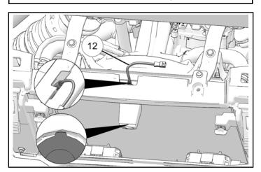
5. Close underhood liner front panel and install two push-pin rivets.
