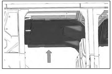
2. Install nine screws in top of roof liner. Torque screws to specification.
