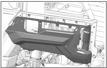
2. Install outer panel with five screws onto vehicle.
