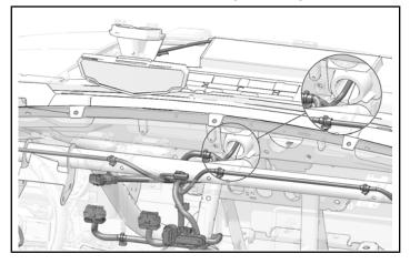
16. Make sure harness 1 connector **2F** is routed through the grommet.
