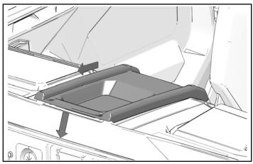
2. Install two push-pin rivets.
