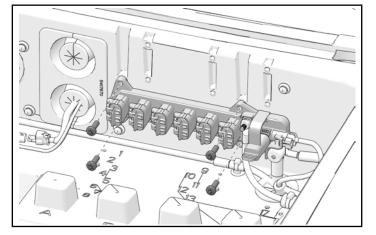
5. Torque Polaris Pulse® bar screws to specification.
