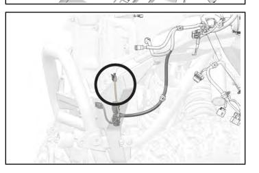
5. Remove cap and connect harness to sensor gauge <sup>(1)</sup>. Make sure to clip any push dart once it is connected.
