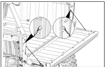
Disconnect dummy connector from vehicle harness. Connect tailgate harness ① connector
