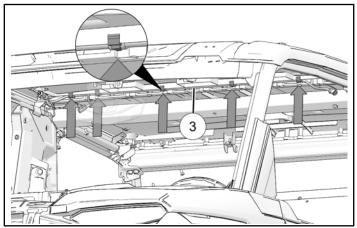
4. Connect rear audio harness connector **4F** to harness ③ connector **4M**.
