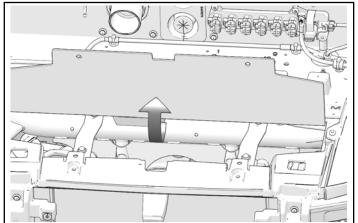
4. Route harness through hole. Look underneath underhood liner if having trouble finding harness. Harness will have a grey connector with purple and brown wires.
