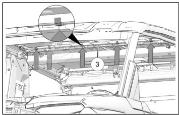
2. Connect harness 3 connector **4M** to vehicle harness.
