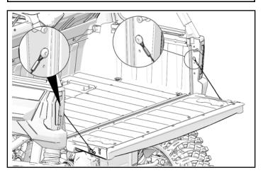
3. Tilt tailgate down and pull left hinge away from vehicle using gap on hinge.
