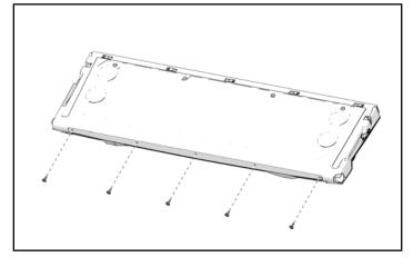
12. Torque five bottom tailgate screws to specification.
