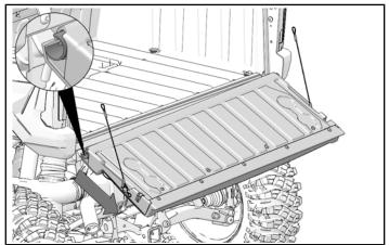
4. Slide right hinge away from vehicle. Remove tailgate from vehicle.
