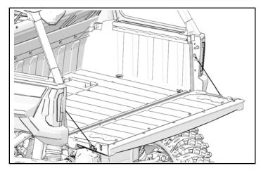
2. Remove left and right tailgate cable from left and right screw.
