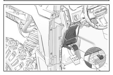
7. Install screw and push-pin rivet in left side door frame.
