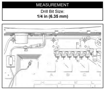
4. Install Polaris Pulse® bar with four kept screws.
