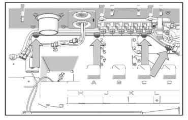
18. Connect harness connector **3M/3F** to winch harness.
