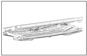
7. Install tailgate harness (2) onto tailgate with three cable ties.
