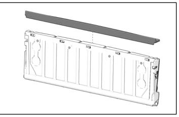
16. Install five kept screws onto tailgate cap.
