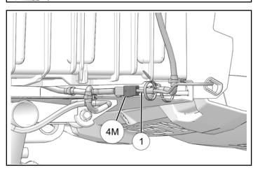
5. Attach tailgate harness to vehicle harness with cable tie.
