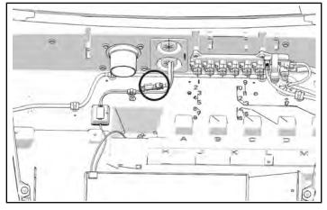
2. Remove harness from vehicle, including edge clips and push darts from center support beam.
