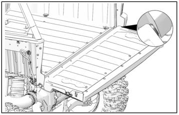
2. Route tailgate harness (2) through left box hinge first. Put left tail gate hinge into box hinge.
