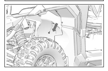
4. Remove five push-pin rivets from bottom of dashboard in front of passenger seat.
