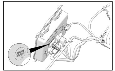
3. Put bottom of head unit into position. Push top of head unit into dash.
