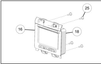
5. Torque four bezel screws (2) to specification.
