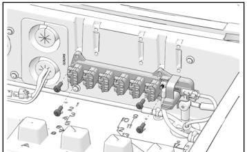
2. Move Polaris Pulse<sup>®</sup> bar with wires forward.
