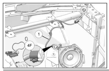
2. Install push-pin rivet at bottom of dashboard in front of drivers seat.
