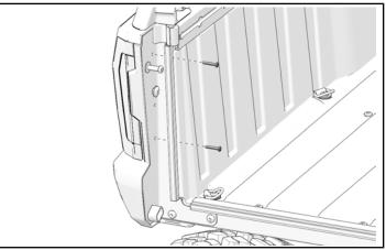
2. Pull tail light and disconnect tail light connection
