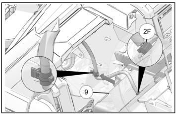
14. Install two push darts onto dash support tube on passenger side. Install edge clip onto plastic chassis.
