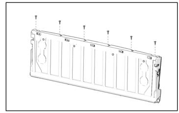
5. Remove and keep five screws from bottom of tail gate assembly.
