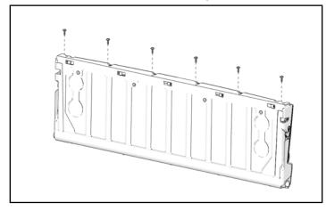
14. Torque top tailgate screws to specification.
