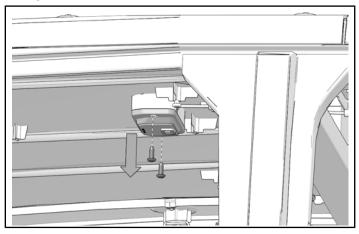
2. Disconnect dome light from wiring harness.
