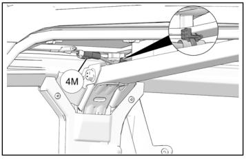
3. Install harness ③ along the back of the roof with five edge clips.
