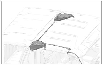
1. Install harness 3 along the roof with five edge clips.
