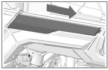
6. Connect tail light to vehicle harness connection. Put tailgate light in place.
