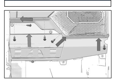
4. Make sure the clip on the dashboard is installed as shown.
