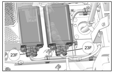
Install edge clip on front close off panel near speaker <sup>(1)</sup>. Connect harness connector **2F** to sub speaker <sup>(1)</sup>.
