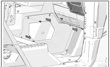
3. Tilt out top of storage panel and remove.
