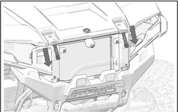
3. Put tabs on grill through openings in front fascia. Push top of grill into proper position.
