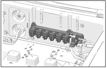
3. Drill three holes as shown. The three holes are dimples. Locations are **1**, **9** and left of **1**.
