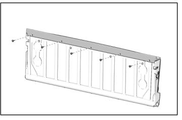
17. Torque five tailgate screws to specification.
