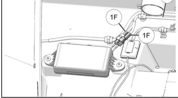
4. Install front camera <sup>(1)</sup> into slot. Make sure the front camera fits into top indent when installing camera.
