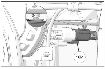
7. Install harness push dart to bracket located at center of dash support tube.
