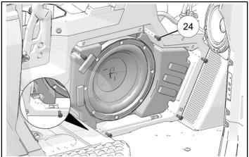
6. Torque screws to specification.
