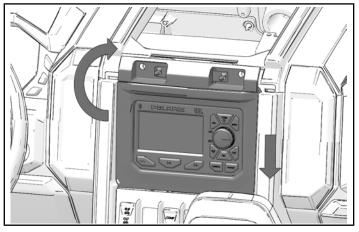
4. Install two push-pin rivets into top of head unit.
