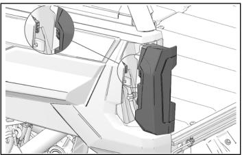
7. Install two tailgate screws into tail gate light. Torque screws to specification.
