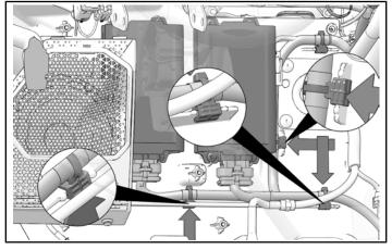
12. Connect harness connector **23F** (Black) and **23F** (White) to both installed amps.
