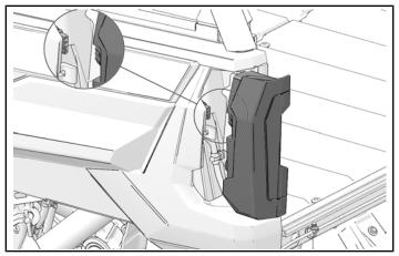
3. Hold down lever and slide upper panel cover to the left to release hooks. Remove upper panel cover from vehicle.
