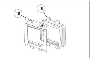
4. Attach bezel display (6) onto dash mount (8) with four bezel screws (2).
