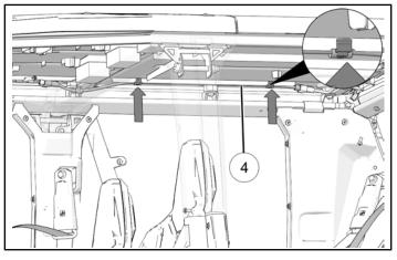
2. Connect rear audio harness connector **4M** to vehicle harness. Attach harness with edge clip as shown.
