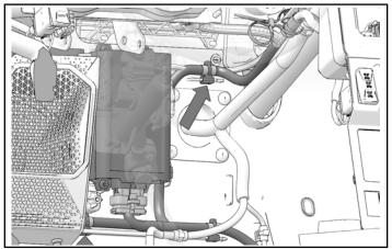
11. Near installed amps, install three edge clips and route harness.
