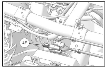
9. Install two push darts onto beam. Install edge clip onto front close-off panel on driver side.
