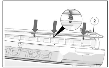
8. Install camera (13). Make sure the camera is aligned with notch in front.
