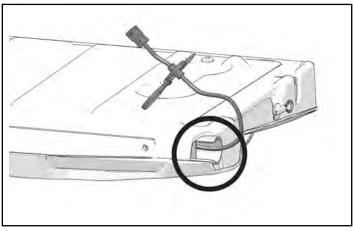
11. Install five kept screws to bottom of tailgate assembly.
