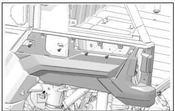
3. Install two bottom outer panel screws
