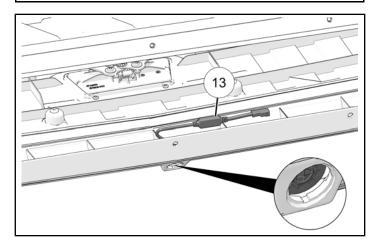
9. Connect camera connector **4M** to tailgate harness connector **4F**.
