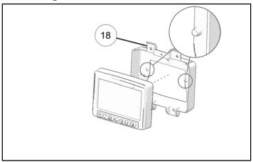
2. Install four u-nuts (2) onto bezel display (6). Make sure the correct side for u-nuts is installed correctly.
