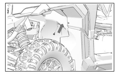
6. Carefully pull trim away from vehicle and install one push-pin rivet in side of dashboard.
