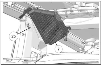
2. Torque audio screws to specification.
