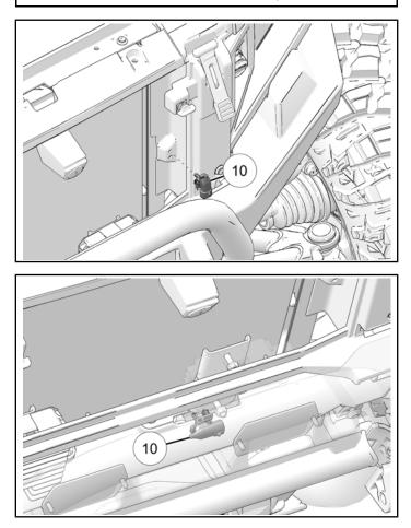
2. Remove two push-pin rivets from the front of the underhood liner.
