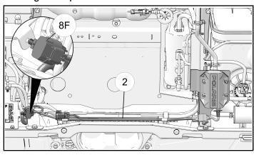
3. Attach harness ② to main wire harness with two cable ties ④.
