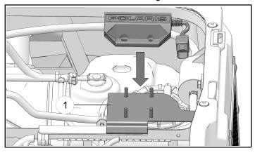
3. Install four nuts **6**. Torque to specification.
