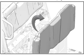
2. Lift seat up and remove from lower hinge brackets.
