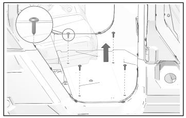
2. Install rail ① and two screws ② in each of the channels. Torque screws to specification.
