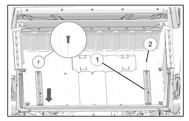
2. Install rail ① and two screws ② in each of the desired locations. Torque screws to specification.
