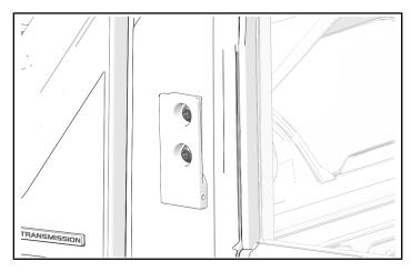
6. Install end cap ① to door mirror assembly ①.
