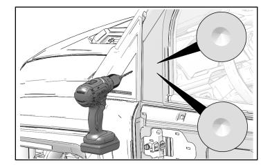
3. Drill holes to expose weld nuts.
