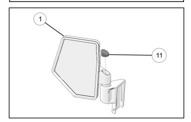
7. Remove adhesive strip and attach foam ① to mirror mount ③.
