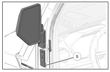
9. Attach assembly to door using screw 9.
