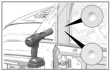
Attach backer plate (5) to door using screws (10).
