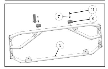
4. Attach plate ® and eight screws ® to mid bed extender frame ⑤. Torque screws to specification.
