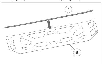
Remove adhesive backing from lower foam ②.
