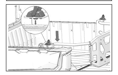
11. Adjust bed extender to desired position. Push down levers on latching assemblies to lock bed extender in place.
