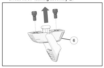
6. Assemble latching assembly to left bed extender frame ③. Torque screws to specification.
