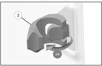
3. Lock four clamps ② to attach panel to ROPS.
