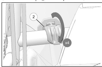
2. Put rear panel ① on vehicle. Make sure bottom edge seats into place on flat area behind seats. Make sure clamps ② are placed against ROPS.
