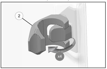
3. Lock four clamps ② to attach windshield to ROPS.
