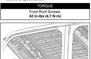
5. ADV models only. Install two kept screws at rear of roof. Torque screws to specification.
