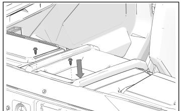
3. If vehicle is equipped with tip-out windshield. Install base, three screws, and washers. Torque screws to specification.
