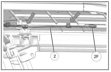
5. Attach harness ④ to harness ②. Route harness ④ across back of roof panel. Attach harness to roof at five locations as shown.
