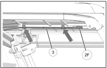
Attach harness ④ to harness ③. Route harness ④ across back of roof panel. Attach harness to roof at five locations as shown.
