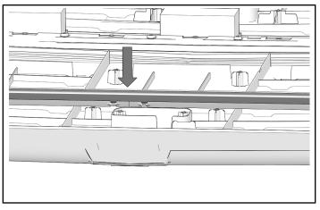
12. Install ten screws to attach seal supports. Torque screws to specification.
