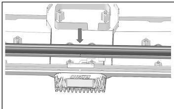
9. Install ten screws to attach seal supports. Torque screws to specification.
