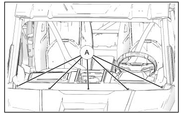
4. Install two push pin rivets on drivers side of dash cover.
