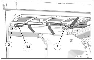
6. Continue routing harness ③ into rear compartment. Attach harness to roof at two points as shown.
