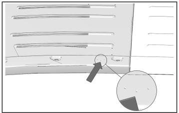
3. Use hole saw to drill large hole at center dimple.
