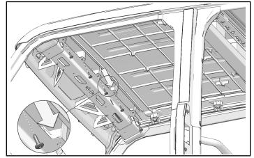
4. Remove and keep two screws from rear underside of roof.
