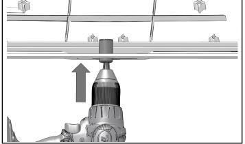
5. Drill holes at screw hole locations. Drill should be perpendicular to outer light mounting surface. Cut through roof panel only.
