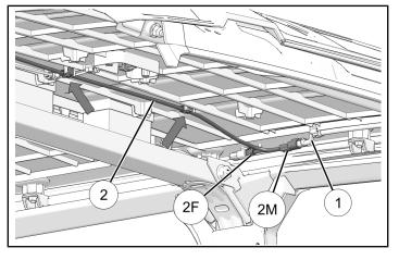
3. Continue routing harness ② across roof. Attach harness to roof as shown. Attach connector **2F** to right scene light.
