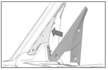
2. Install three screws. Torque to specification.
