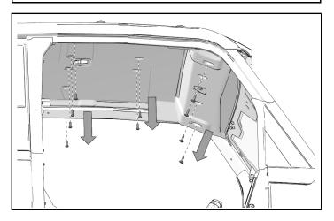
6. Remove and keep front roof liner.
