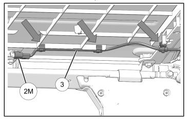
6. Route harness ③ across roof. Attach harness to rear cap at two points as shown.
