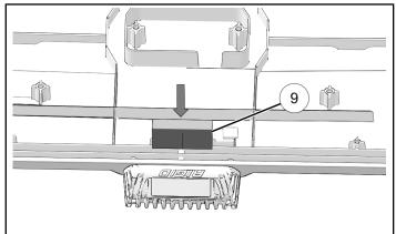
8. Install roof seal and supports in correct position.
