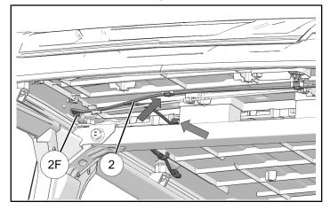
4. Continue routing harness ② along rear roof panel. Attach harness ③ at two points as shown.
