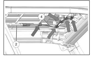
6. Attach remaining connector on harness ④ to rear scene light.
