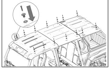
4. Install five kept screws at front of roof. Torque screws to specification.
