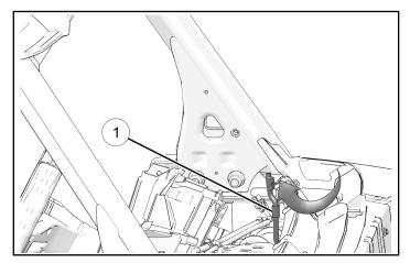
4. Route wiring harness through ROPS A-pillar while watching for end to appear in opening above drivers window area.
