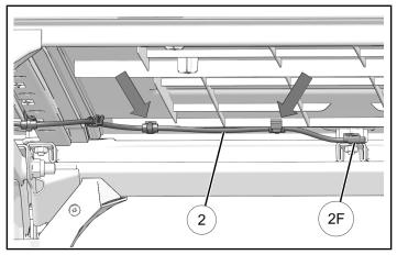
5. Attach connector **2M** of extension harness ③. Route harness ③ toward rear of vehicle. Attach harness to roof at three points as shown.
