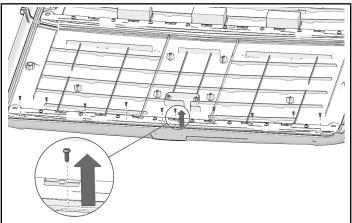
3. Pull up on seal and seal supports at rear of roof. Hold up seal to prevent damage during drilling.
