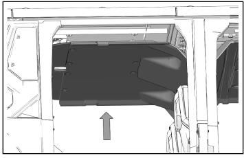
2. Install nine screws in top of roof liner. Torque screws to specification.
