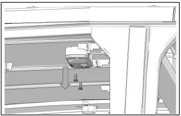
3. Disconnect dome light from wiring harness.
