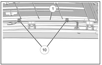
Attach connector 2M of scene light harness (2) to harness (1). Attach connector 2F to left scene light. Route harness toward right side of vehicle. Attach harness clips to roof at two points as shown.
