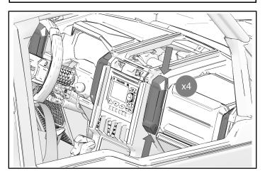
2. Remove one screw at each side of dash cover.
