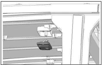
4. Remove and keep nine screws from mid roof liner.
