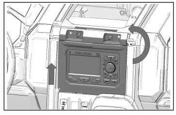
3. Disconnect wiring harness and antenna from head unit. Remove head unit.
