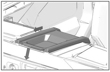
2. Install two push-pin rivets.
