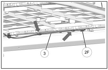
7. Attach remaining connector from harness ③ to rear scene light.
