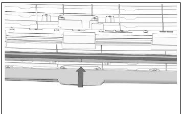
4. Find three dimples at center rear of roof. Use hole saw to drill large hole at center dimple. Hole saw should be perpendicular to outer light mounting surface. Cut through roof panel and two support ribs.
