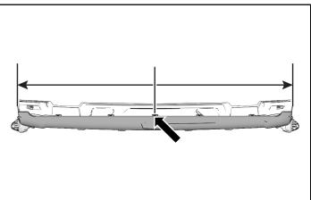
5. Measure from bottom edge of roof at center point to determine center drill location. Mark this location.
