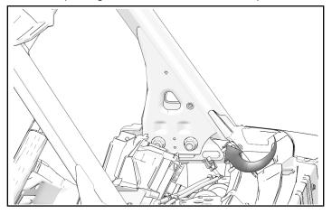
3. Route end of harness ① up into opening in ROPS A-pillar.
