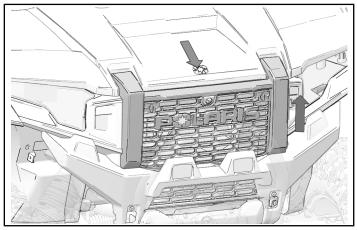
3. Pull rubber straps off hooks to release hood. Lift hood to remove.
