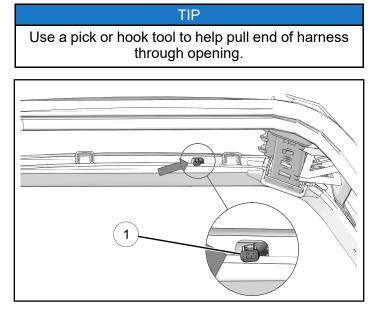
6. Attach connectors on lower end of harness ① into mounts on frame.
