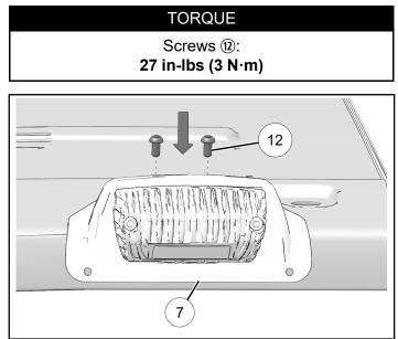
8. Pull down on pod so that pod contacts roof panel over entire bottom surface. Continue pulling down while drilling bottom holes.
