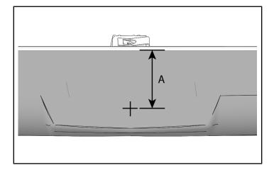
6. Measure on either side of center point and from bottom edge to find screw hole locations. Mark these locations.
