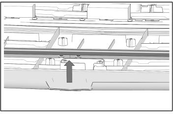
4. Measure width of rear roof cap. Mark center of cap.
