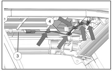
8. Attach remaining connector on harness ④ to rear scene light.
