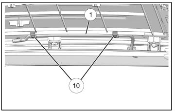
Attach connector 2M of scene light harness 1 to harness 1. Attach connector 2F to left scene light. Route harness toward right side of vehicle. Clip harness to roof at two points as shown.
