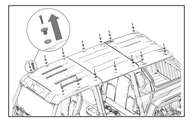
3. Remove and keep five screws from front underside of roof.
