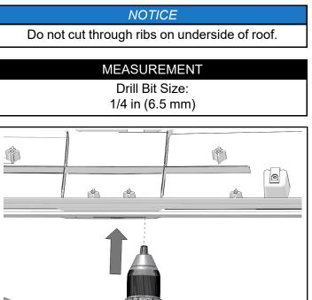
Install scene light (5) on roof. Wiring harness from light will pass through large hole in roof. Use two screws (1) and two nuts (3) to attach light. Torque nuts (3) to specification.
