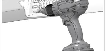
10. Install two screws <sup>(1)</sup> in bottom holes of pod. Torque screws to specification.
