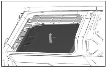
2. Install eight screws in roof liner. Torque screws to specification.
