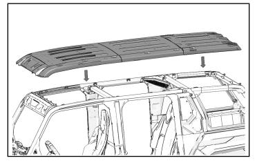
3. Install kept screws, spacers, and washers to attach roof. Torque screws to specification.
