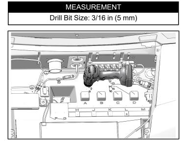
10. Pull end of harness ① containing fuse block and Pulse<sup>®</sup> connector through top of grommet to hood area. Push harness clip into hole at location **7**. Push fuse block clip into hold at location **A**. Connect harness to Polaris Pulse<sup>®</sup> bar.
