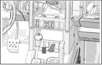
12. Route harness ① behind switch panel. Pull switch connector through opening.
