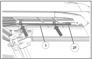
7. Attach harness ④ to harness ③. Route harness ④ across back of roof panel. Attach harness to roof at five locations as shown.
