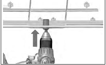
5. Drill holes at screw hole locations. Drill should be perpendicular to outer light mounting surface. Cut through roof panel only.
