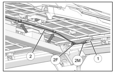
3. Continue routing harness ② across roof. Attach harness to roof as shown. Attach connector **2F** to right scene light. Route remaining leg of harness over ROPS. Attach edge clip to roof as shown.
