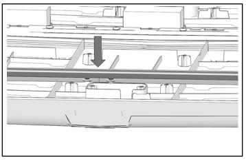
12. Install ten screws to attach seal supports. Torque screws to specification.
