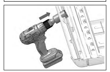
8. Drill holes at screw hole locations. Drill should be perpendicular to outer light mounting surface. Cut through roof panel only.
