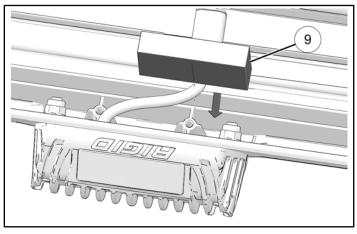
11. Install roof seal and supports in correct position.
