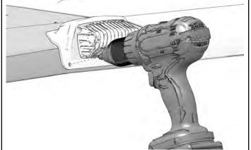
10. Install two screws <sup>(1)</sup> in bottom holes of pod. Torque screws to specification.
