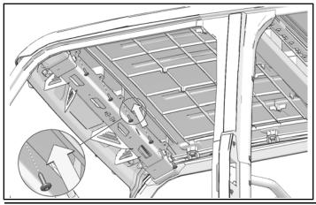
5. ADV models only. Install two kept screws at rear of roof. Torque screws to specification.
