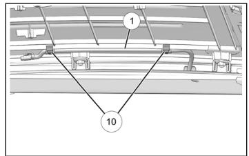
Attach connector 2M of scene light harness 2 to harness 1. Attach connector 2F to left scene light. Route harness toward right side of vehicle. Attach harness to roof at two points as shown.
