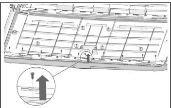
Pull up on seal and seal supports at rear of roof. Hold up seal to prevent damage during drilling.
