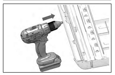
Install scene light (5) on roof. Wiring harness from light will pass through large hole in roof. Use two screws (1) and two nuts (3) to attach light. Torque nuts (3) to specification.
