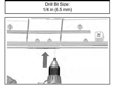
Install scene light (5) on roof. Wiring harness from light will pass through large hole in roof. Use two screws (1) and two nuts (3) to attach light. Torque nuts (3) to specification.
