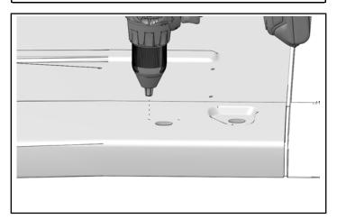
5. Remove backing from gasket (8). Install gasket on bottom side of scene light pod ①.
