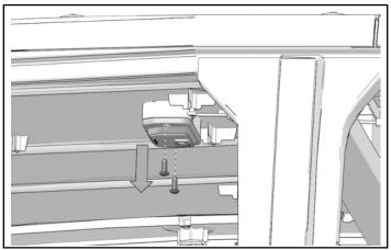
3. Disconnect dome light from wiring harness.
