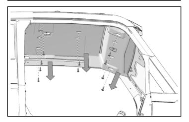
6. Remove and keep front roof liner.
