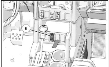
15. Use cable tie on harness ① to attach harness to existing harnesses behind head unit opening, as shown.
