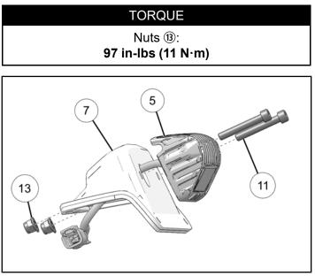
7. Install two screws (1) at top of pod (7). Torque screws to specification.
