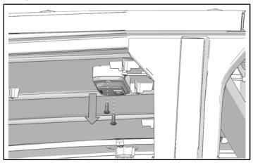
2. Disconnect dome light from wiring harness.
