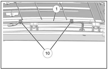
Attach connector 2M of scene light harness (2) to harness (1). Attach connector 2F to left scene light. Route harness toward right side of vehicle. Clip harness to roof at two points as shown.
