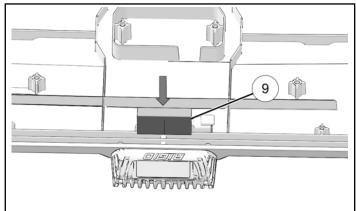
8. Install roof seal and supports in correct position.
