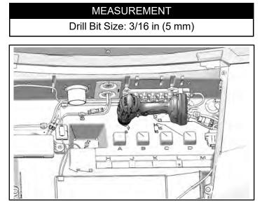
Pull end of harness ① containing fuse block and Pulse<sup>®</sup> connector through top of grommet to hood area. Push harness clip into hole at location 7. Push fuse block clip into hold at location A. Connect harness to Polaris Pulse<sup>®</sup> bar.
