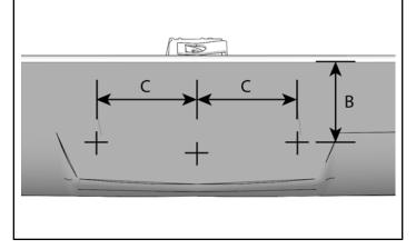
7. Use hole saw to drill large hole at center location. Hole saw should be perpendicular to outer light mounting surface. Cut through roof panel and two support ribs.
