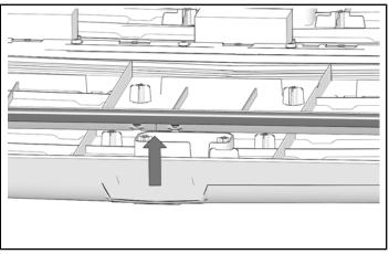
4. Measure width of rear roof cap. Mark center of cap.
