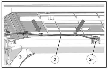
5. Attach connector **2M** of harness ③ to harness ②. Route harness ③ toward rear of vehicle, passing over ROPS. Attach harness to roof at three points as shown.
