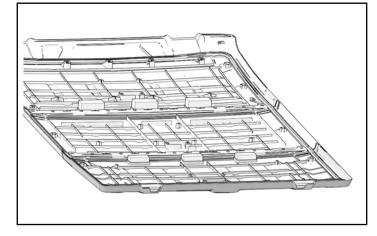
2. Remove and keep ten screws from seal support panels.
