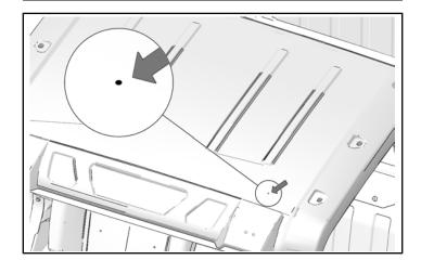
3. Lightbar kit will contain a grommet. Measure grommet to determine needed hole size.
