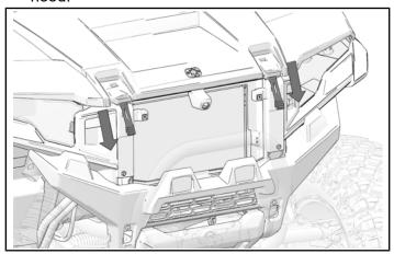
3. Put tabs on grill through openings in front fascia. Push top of grill into correct position.
