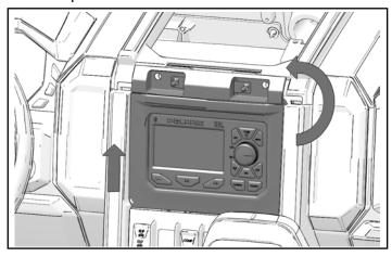
Disconnect wiring harness and antenna from head unit. Remove and keep head unit.
