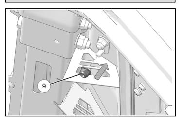
6. Remove the other nut from the original mounting hardware.
