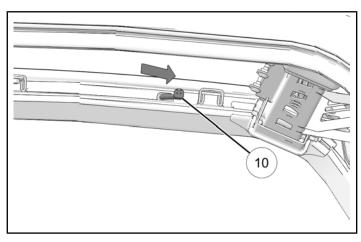
6. Pull harness through A-pillar until connectors at the dashboard end of the harness line up with positions shown. Secure harness (1) to frame with push-dart clips.
