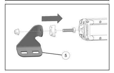
For 33 inch lightbar, assemble bracket ⑤ and bracket ⑥ to lightbar. Use screw, lockwasher, and washer from lightbar kit. Tighten screw until fully seated.
