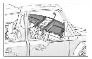
If vehicle is equipped with upper tweeters, make sure to unplug tweeters when removing dash cover.
