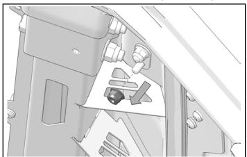
3. Remove one screw from upper hinge.
