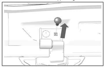
4. Install carriage screw ①, tubular spacer ②, washer plate ③, 3mm spacer ⑦, and bracket ⑤. Rotate washer plate so that the other screw can be removed later. Tubular spacer will pass through the hole drilled in roof.
