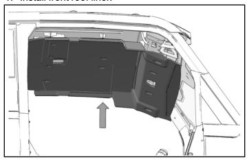
2. Install six screws in top of roof liner and four screws in front of roof liner. Torque screws to specification.
