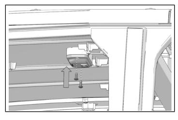
5. Install rearview mirror assembly with two screws. Torque screws to specification.
