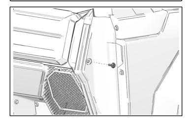
3. Carefully pull plastic cover away from lower A-pillar area and remove one push-pin rivet from side of dash cover.
