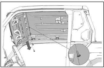
2. Remove and keep three front screws, spacers, and washers from each side of roof.
