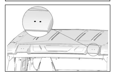
2. Locate drill point for grommet behind the drivers side eyebrow feature. Drill pilot hole at this location.
