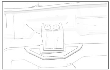
2. Remove one nut from upper clamp mounting.
