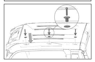
4. Install five screws in underside of roof. Torque screws to specification.
