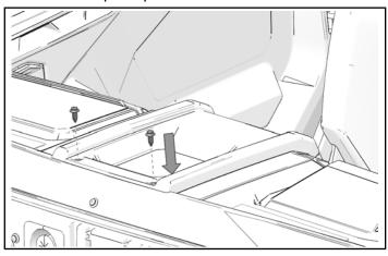
3. If vehicle is equipped with tip-out windshield. Install base, three screws, and washers. Torque screws to specification.
