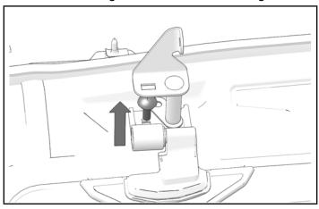
8. Rotate washer plate ③ to line up with the remaining hole.
