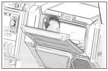
5. Remove and keep five screws (A) and washers at front of dash cover.
