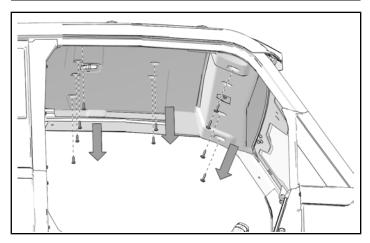
6. Remove and keep front roof liner.
