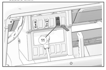
12. Attach harness to mounting point behind head unit opening as shown.
