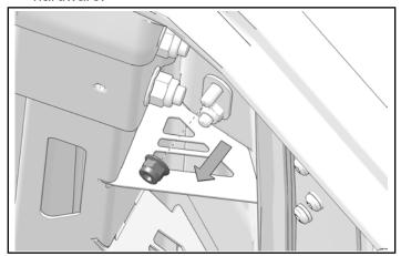
7. Remove carriage screw from window clamp.
