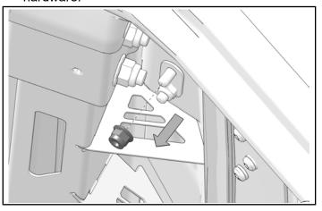
7. Remove carriage screw from window hinge.
