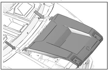
2. Pull rubber straps down over hooks to secure hood.
