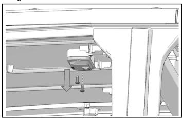
3. Disconnect dome light from wiring harness.
