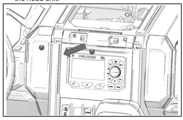
2. Pull top of head unit away from dash and lift head unit up to remove from dash.
