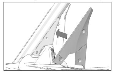
2. Install three screws. Torque to specification.
