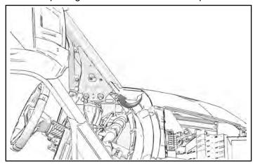
3. Feed end of harness (1) shown up into opening in ROPS A-pillar.
