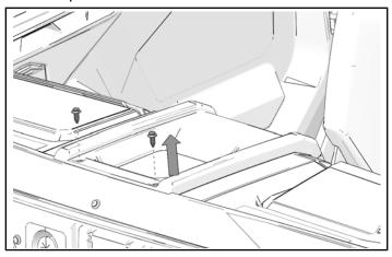
2. Remove and keep panel by lifting front edge and moving backward.
