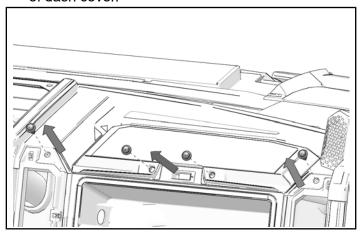
7. Remove two push-pin rivets from drivers side of dash cover.
