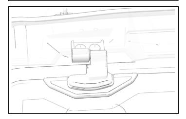
2. Remove one nut from upper hinge mounting.
