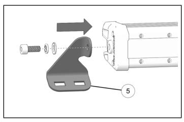
For 40 inch lightbar, assemble bracket (1) to each end of lightbar. Use screw, lockwasher, and washer from lightbar kit. Tighten screw until fully seated.
