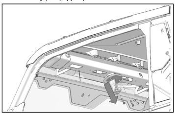
2. Remove and keep two screws to uninstall dome light.
