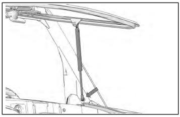
4. Remove two screws and ball stud from lower A-pillar trim panel.
