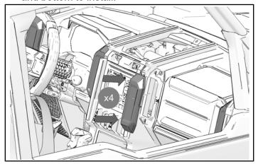
7. Install one push pin rivet at each side of dash.
