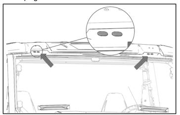
2. Install bracket ⑤, two carriage screws ①, two tubular spacers ②, 3 mm spacers ⑦, and 5 mm spacers ⑧ at the eyebrow feature.
