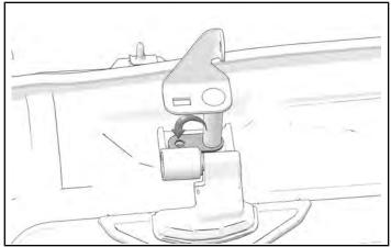
9. Install carriage screw 1 , tubular spacer 2, and 3mm spacer 1.
