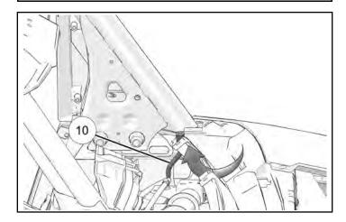
4. Feed wiring harness through ROPS A-pillar while watching for end to appear in opening above drivers window area.
