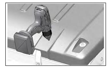
3. Find grommet drill point in front of dimples. Drill pilot hole at this location.
