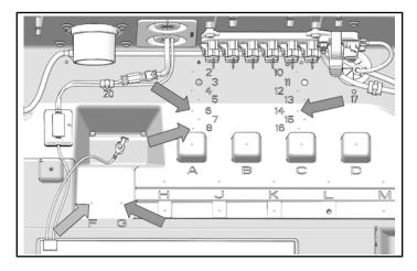
Install plow angle control harness ①. Install relays at locations F and G. Install fuse holder at location 8. Install harness push dart clips at locations 6 and 14. Plug harness into Polaris Pulse® bar.
