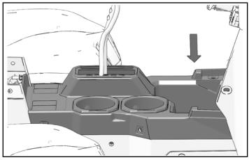
2. Install four push-pin rivets to assemble cover to base.
