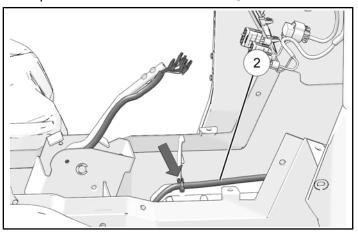
2. Route harness ② through shifter mounting bracket, as shown. Use edge clips to attach harness to mounting bracket in three locations.
