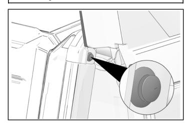
8. Install one screw at each side of dash. Torque to specification.
