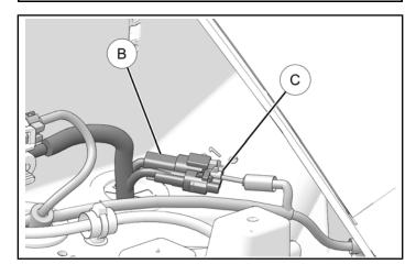
Install connector 4F of harness ② into connector from winch harness ③. Install connector 4M of harness ② into connector from chassis harness ⑥.
