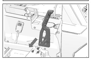
4. Remove and keep four push-pin rivets from cover.
