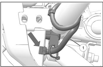
7. Connect harness ① to harness from tilt actuator.
