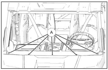
6. Remove four push-pin rivets from passenger side of dash cover.
