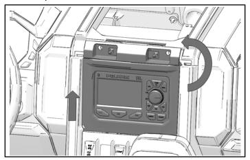
3. Disconnect wiring harness and antenna from head unit. Remove and keep head unit.
