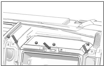
6. Install four dash vent covers. Push evenly at top and bottom to install.
