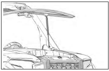
2. Remove and keep three screws and washers. Remove and keep windshield base.
