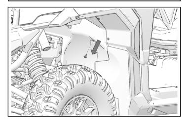
4. Remove five push-pin rivets from bottom of dashboard in front of passenger seat.
