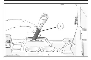
11. Install new shifter boot <sup>®</sup> into cover. Thicker side of boot should be toward left side. Thinner side should be toward right side.
