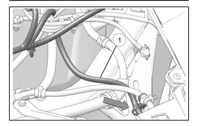
5. Continue routing harness ① toward bottom of front lower fascia. Use cable tie to attach harness as shown. Wrap harness around bumper support tube as shown.
