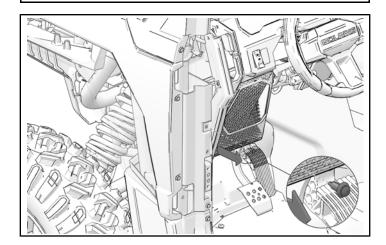
3. Remove one screw from each front wheel well.
