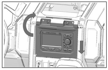
3. Install two push-pin rivets into top of head unit.
