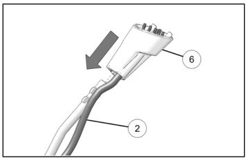
5. Use previously removed screw to assemble knob base **(6)** to shift handle.
