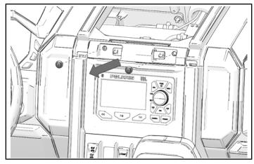
2. Pull top of head unit away from dash and lift head unit up to remove from dash.
