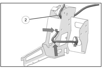
3. Route longer end of harness ② under dash area, through bottom half of grommet, and into underhood area.
