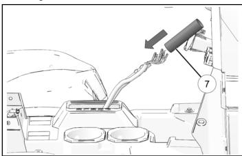
4. Install harness ② through hole in knob base ⑥. When harness is in correct position, install knob base on shift lever.
