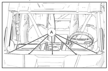
4. Install two push pin rivets on drivers side of dash cover.
