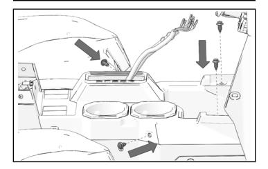
3. Install heat shrink tube ① around handle and wiring harness.
