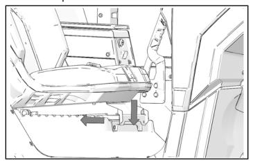
2. Install two kept screws at front of seat base. Torque screws to specification.
