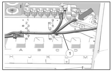
4. Route harness ① under liner and use cable tie to attach harness as shown.
