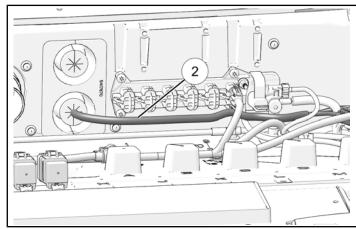
4. Location connection between winch harness ® and chassis harness © in underhood harness. Separate these connectors.
