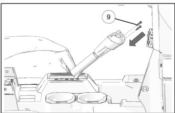
10. Push heat shrink tube ① down to base of shift lever. Make sure harness is routed on right side of shift lever. Use heat gun to shrink tube in place around lever and harness.
