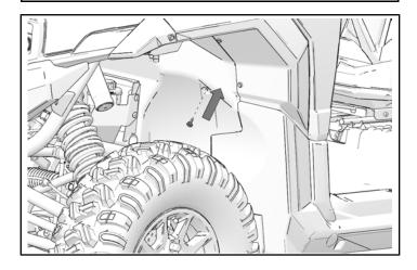
6. Carefully pull trim away from vehicle and install one push-pin rivet in side of dashboard.
