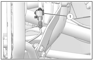
8. When plow is not in use, install tilt harness connector into cap attached to harness ①.
