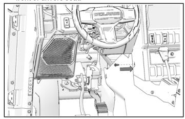
3. Install five push-pin rivets at bottom of dashboard in front of passenger seat.
