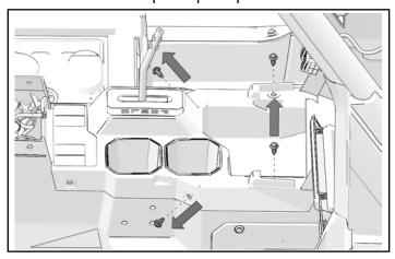
5. Place shift lever in NEUTRAL position. This will aid removal and later installation.
