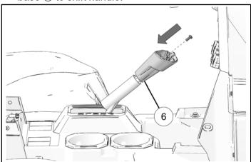
6. Install switches ③ into shift knob cap ④. If there are positions which will not have a switch, install filler plug ⑤ instead.
