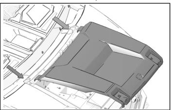
Pull rubber straps down over hooks to secure hood.
