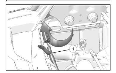
4. Feed wiring harness through ROPS A-pillar while watching for end to appear in opening above passenger window area.
