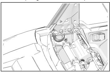
3. Feed end of harness ① shown up into opening in ROPS A-pillar.
