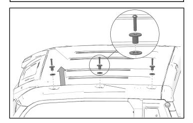
3. Remove and keep three weld nuts from each side of roof underside.
