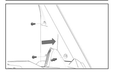
3. Return clip at bottom of gas spring to engaged position. Connect bottom of gas springs.
