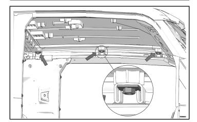
3. Install three washers, spacers, and screws on each side of roof. Tighten screws to specification.
