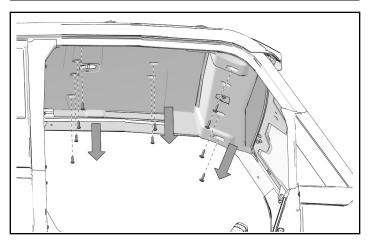
6. Remove and keep front roof liner.
