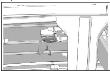
3. Disconnect dome light from wiring harness.
