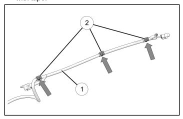
9. While holding ROPS harness ① in position, press first clip ② into recessed part of roof strengthening rib. Press last clip into roof strengthening rib so dome light wiring is positioned in recessed part of rib. Press middle clip onto roof strengthening rib. Tighten cable ties.
