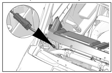
2. Put front of dash cover in position and set into place. Make sure center of dash is placed in slots on vehicle.
