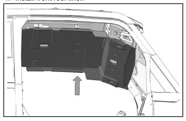
2. Install six screws in top of roof liner and four screws in front of roof liner. Torque screws to specification.
