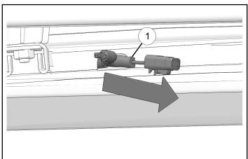
6. Pull ROPS harness through opening until push dart clips on dash end of harness line up with positions shown. Secure ROPS harness ① in positions shown using push pin clips. Connect ROPS harness to main vehicle harness.
