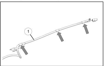
8. Loosely install three edge clips ② in spots marked with tape.
