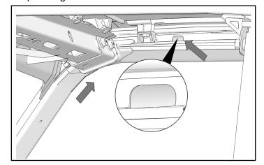
5. Pull end of ROPS harness ① through opening in ROPS.
