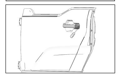
2. Install key core ② in the actuator assembly.
