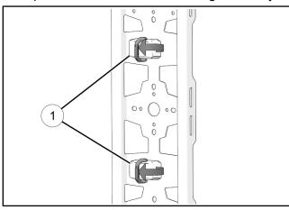
2. Install plate-tool mount rack ② onto main bed rack by aligning latching assembly ① with openings in box rail and install onto rail.
