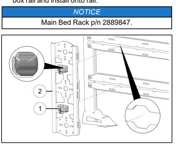
3. Close latching assembly ① to lock in place.
