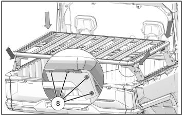
8. Torque screws (8) and (9) using included tool as needed.
