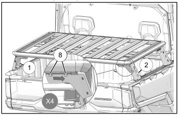
7. Install two screws (8) into each brace.
