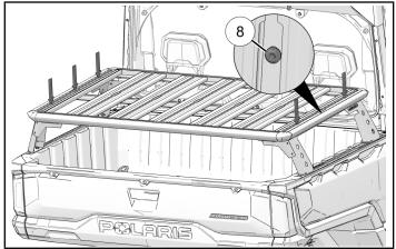
6. Loosen screws (3) on front and rear braces. Slide outward until holes line up with matching holes on backbones (1) and (2).
