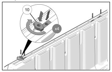
2. Put backbone ① on box rail. Loosely install four screws ⑨ into installed T-nuts ⑩.
