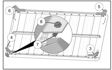
4. Put rack on installed backbones ① and ②.
