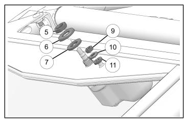
4. Install cap ® over nut on arm stopper shaft. Install wiper arm cap ④ onto wiper arm shaft.
