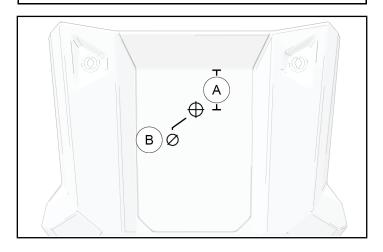
2. Pass nozzle ③ through hood panel and secure with nozzle nut.
