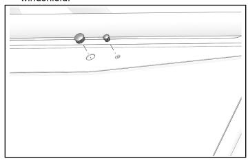
2. Slide the following hardware onto wiper arm shaft and arm stopper shaft.
