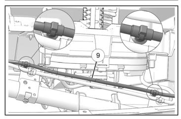
Pull end of harness (1) containing fuse block, relay, and Pulse<sup>®</sup> connector through grommet to hood area. Push harness push darts into holes at locations 3 and 11. Install push dart for relay into hole at position L. Connect harness to Polaris Pulse<sup>®</sup> bar.
