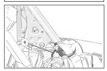
4. Feed wiring harness through ROPS A-pillar while watching for end to appear in opening above drivers window area.
