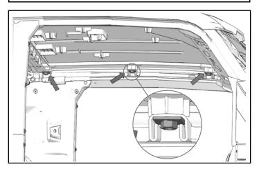
3. Install three washers, spacers, and screws on each side of roof. Tighten screws to specification.
