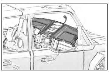
9. If vehicle is equipped with upper tweeters, make sure to unplug tweeters when removing dash cover.
