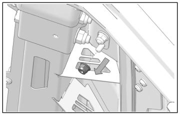
3. Remove one screw from upper hinge.
