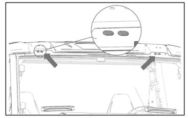
Install bracket (4), two carriage screws (1), two tubular spacers (2), 3 mm spacers (5), and 5 mm spacers (6) at the eyebrow feature.
