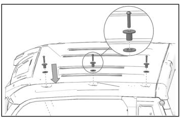
4. Install five screws in underside of roof. Torque screws to specification.
