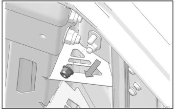
7. Remove carriage screw from window clamp.
