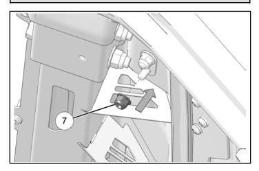
6. Remove the other nut from original mounting hardware.
