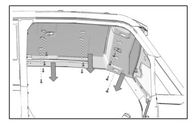
6. Remove and keep front roof liner.
