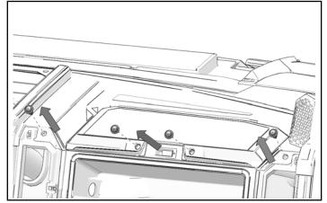
7. Remove two push-pin rivets from drivers side of dash cover.
