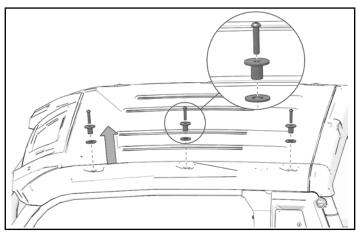
3. Remove and keep three weld nuts from each side of roof underside.
