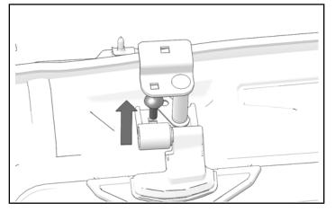
8. Rotate washer plate ③ to line up with remaining hole.
