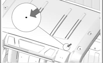
3. Cube light kit will contain two grommets. Measure grommet to determine needed hole size.
