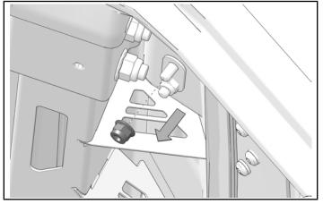
7. Remove carriage screw from window hinge.
