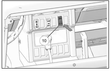
12. Clip harness to mounting point behind head unit opening as shown.
