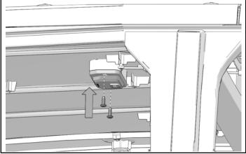
5. Install rearview mirror assembly with two screws. Torque screws to specification.
