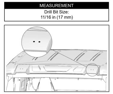
2. Locate drill point for grommet behind drivers side eyebrow feature. Drill pilot hole at this location.
