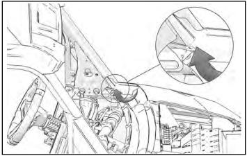
3. Feed end of harness (9) shown up into opening in ROPS A-pillar.
