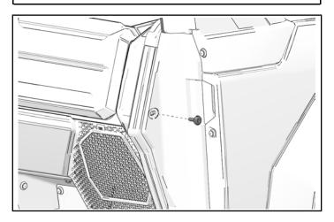
3. Carefully pull plastic cover away from lower A-pillar area and remove one push-pin rivet from side of dash cover.
