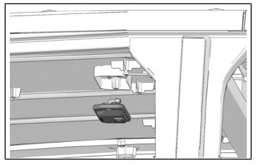
5. Remove and keep six screws from top of roof liner and four screws from front of roof liner.
