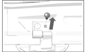
Install carriage screw ①, tubular spacer ②, washer plate ③, 3 mm spacer ⑤, and bracket ④. Rotate washer plate so that the other screw can be removed later. Tubular spacer will pass through hole drilled in roof.
