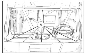
4. Install two push pin rivets on drivers side of dash cover.
