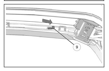
6. Pull harness through A-pillar until connectors at dashboard end of harness line up with positions shown. Secure harness (1) to frame with push darts.
