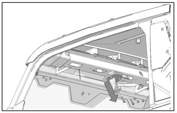
2. Remove and keep two screws to uninstall dome light.
