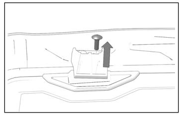
Install carriage screw ①, tubular spacer ②, washer plate ③, and bracket ④. Rotate washer plate so that the other screw can be removed later. Tubular spacer will pass through hole drilled in roof.
