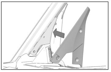
2. Install three screws. Torque to specification.
