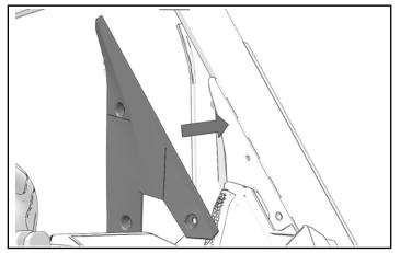
2. Install two screws and ball stud. Torque to specification.
