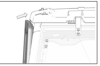
3. Turn handles upward to lock window into place.
