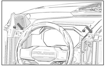
5. Install four push pin rivets on passenger side of dash cover.
