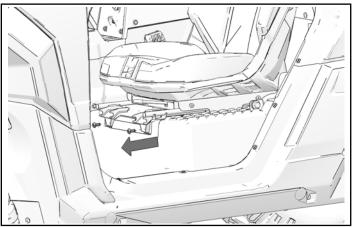
2. Lift front of seat and pull forward to remove seat.
