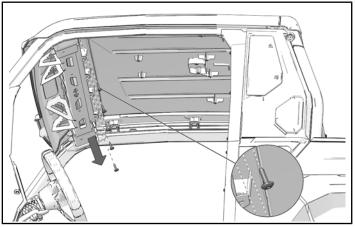
2. Remove and keep three front screws, spacers, and washers from each side of roof.
