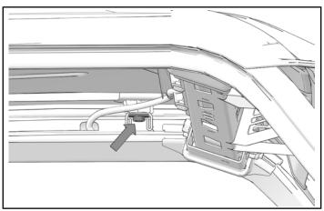
Position lightbar ① on roof. Install washer ④ between lightbar mount and T washer. Install screw ③ into roof screw hole.
