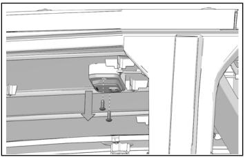
3. Disconnect dome light from wiring harness.
