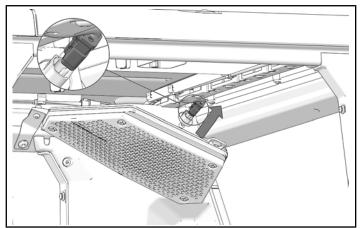
2. Remove and keep two screws. Remove the speaker.
