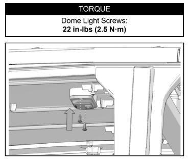
5. Install rearview mirror assembly with two screws. Torque screws to specification.
