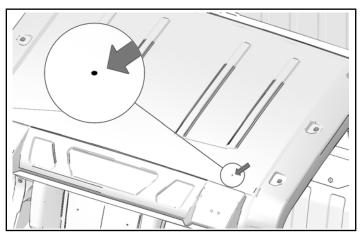
4. Lightbar kit will contain a grommet. Measure grommet to determine needed hole size.
