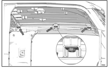
4. Use bar or other appropriate object to prop up corner of roof.
