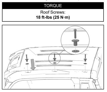
4. Install five screws in underside of roof. Torque screws to specification.
