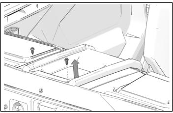
2. Remove and keep panel by lifting front edge and moving backward.
