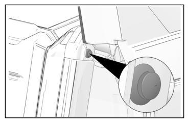
8. Install one screw at each side of dash. Torque to specification.
