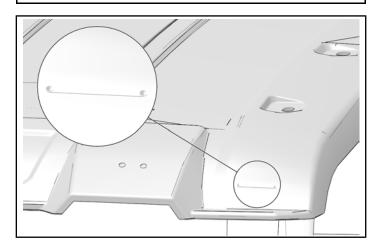
3. Locate drill point for grommet behind drivers side eyebrow feature. Drill pilot hole at this location.
