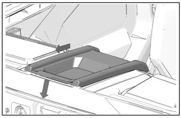
2. Install two push-pin rivets.
