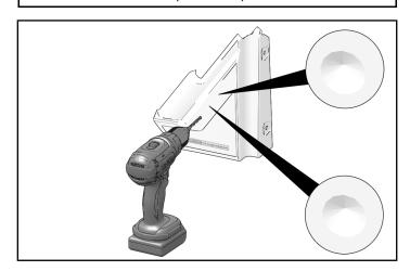
4. Loosely install two screws ① into bracket ⑤ to align it properly.
