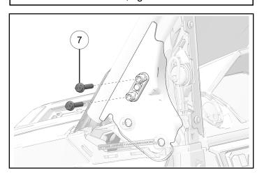
8. Install A-pillar cover using two kept push-pin rivets, make sure A-pillar cover tabs engage body plastic.
