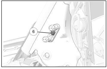
7. Remove and keep two screws ① from bracket assembly.
