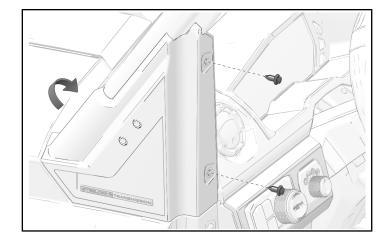
9. Install mirror assembly 1 to bracket using two screws 2.
