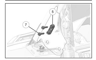
5. Install bracket ⑤ to vehicle frame using one screw
