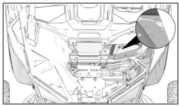
2. Disconnect connector from plug cap. Remove plug cap from vehicle.
