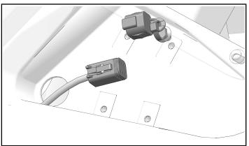
Install RIDE COMMAND+ Plug-In and four screws
