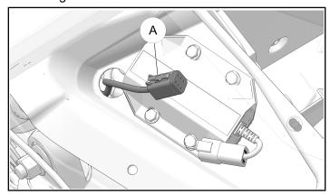
6. Connect main wire harness connector (A) to RIDE COMMAND+ Plug-In connector.
