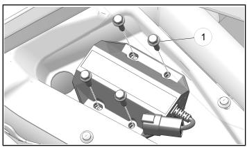
4. Install four screws ① with four nuts ②. Torque nuts to specification.
