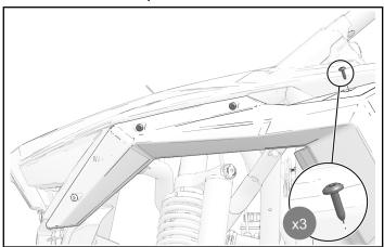
3. Remove and keep three hood fasteners.
