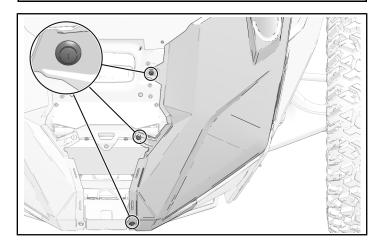
2. Install three retained front fender fasteners. Torque fender fasteners to specification.
