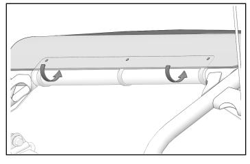
7. Loosely install three screws ④, retained washers and nuts through roof panel, poly rear panel and existing P-clamps.
