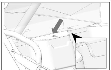
6. Fit top edge of poly rear panel under existing roof panel.
