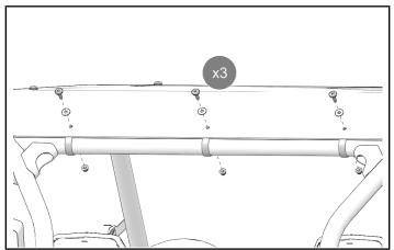
2. Install three P-clamps on ROPS bar. Make sure flat part of P-clamp is positioned to toward rear of vehicle and mounting hole is positioned down.
