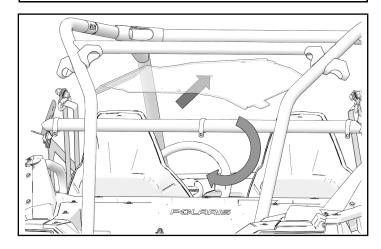
5. Fit tabs on bottom edge of poly rear panel in front of panel at rear of rider compartment. Center section of panel should rest on top of rear panel section of rider compartment.
