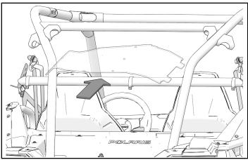
4. Lift and turn poly rear panel while pulling back into position on rear of ROPS.
