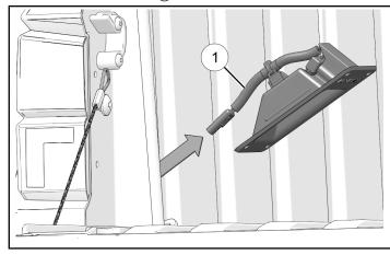
23. Install 12V Accessory box assembly using screws ①. Torque until fully seated.
