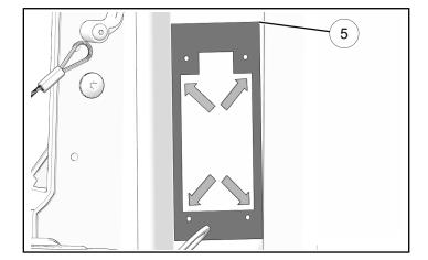
22. Route end of harness ② (not shown) with connector **2F** under cargo box and through hole. Connect to cable ①.
