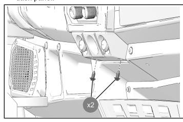
4. Pull center dash panel down, then away from dash to gain access to harness.
