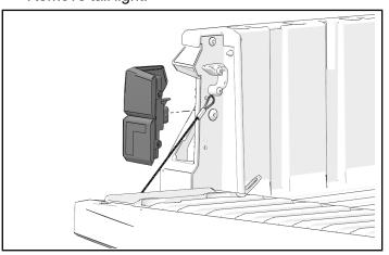
19. Install template ⑤ in left rear corner of cargo box. Make sure side and bottom of template line up with contours in corners of box. Mark cutout edges and hole locations using scribe tool or paint marker.
