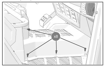
2. Install two fasteners located under seat area.
