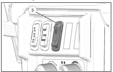
7. Install center dash panel. Lift into place. Make sure two retainer tabs at top of panel engage in slots.
