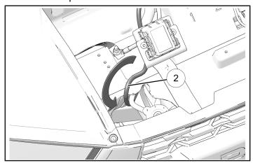
10. Route harness ② along frame. Attach using cable ties
