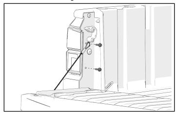
18. Pull tail light out of opening and disconnect wiring. Remove tail light.
