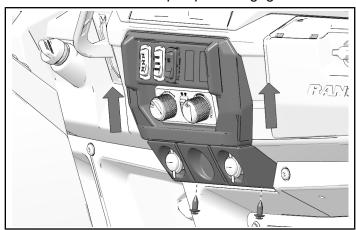
8. Install two push pin rivets.
