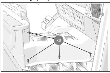
2. Remove two fasteners located in under seat/storage bin area. Remove tunnel cover.
