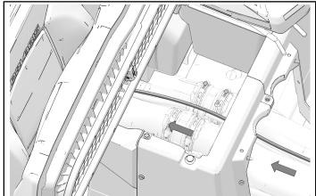
12. Route harness toward rear of vehicle. Attach to existing wiring using cable ties.
