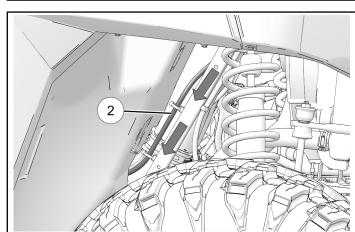
11. Route harness along center hump as shown. Attach to existing wiring using cable ties.
