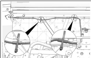
14. Make sure harness ② is routed away from hot or moving parts. Make sure harness is attached using cable ties.
