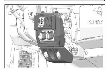
5. Pull connector **12F** through switch hole in dash and connect to 12V switch ③.
