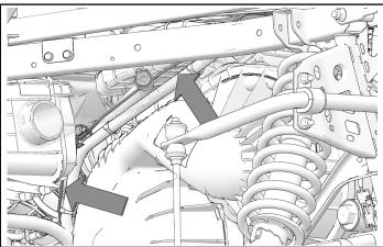
13. Route harness ② along taillight wiring. Attach with cable ties.
