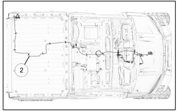
15. Route harness ② along tail light wiring at center of vehicle and over to left tail light area.
