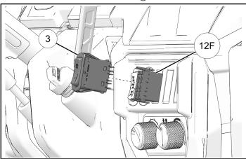
6. Install switch ③ in switch hole opening. Push until it clicks into place.
