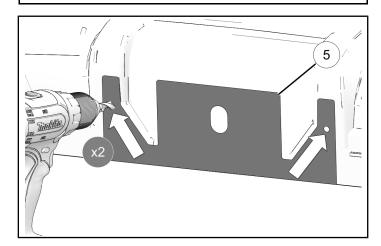
4. Cut middle opening using a utility knife or similar. Remove template when complete.
