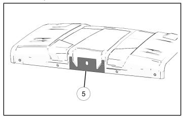
2. Mark drill positions and cutout position. Make sure drill positions are marked in the center of the hole.
