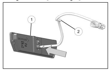
8. Install worklight ① onto bezel. Route wiring through center opening. Install using screws ⑥. Torque until fully seated.
