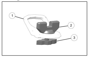
2. Insert the T-nut through one of the port openings in the rail. Slide clamp assembly to the desired location on the rail. Tighten wing screw until fully clamped.
