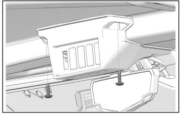
3. Remove two screws from middle of front roof liner. If equipped with dome light, remove dome light and disconnect any wiring.
