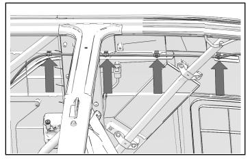
4. Install four edge clips near rear end of roof.
