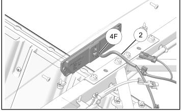
3. Install two screws (4) into rear work light (1). Torque screws to specification.
