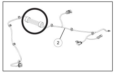
2. Install three edge clips near front of roof. Make sure harness ② connector **10F** is located near the front.
