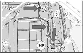
3. Install four edge clips along roof.
