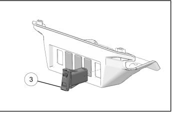
3. Put switch panel near rear work light harness ② connector **10F**. Connect work light harness ③ connector **10F** to work light switch ③.
