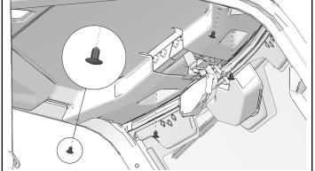
3. If vehicle is equipped with dome light, connect dome light and install onto roof liner with two screws. Torque two screws to specification
