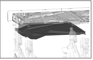
2. Install two screws (A) and four push dart clips into rear roof liner.
