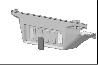
2. Install rear work light switch ③ into switch panel slot.
