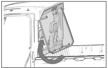
2. Put rear panel mounts onto the cab frame.
