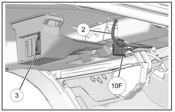
4. Install switch panel to roof using two push-pin darts and two screws. Torque screws to specification.
