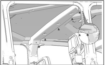
5. Three-passenger Model Only: Install two screws and two push dart clips from rear of front liner. Torque screws to specification.
