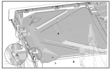
2. Remove rear roof liner from roof.
