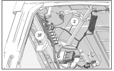
5. Attach harness ② fuse connector **2F** to roof hole with push dart clip.
