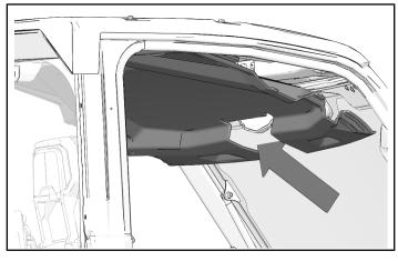
2. Install four push dart clips at front of roof liner.
