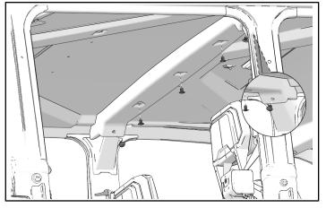
5. Three-passenger Vehicle Only: Remove two screws and two push dart clips from rear of front liner.
