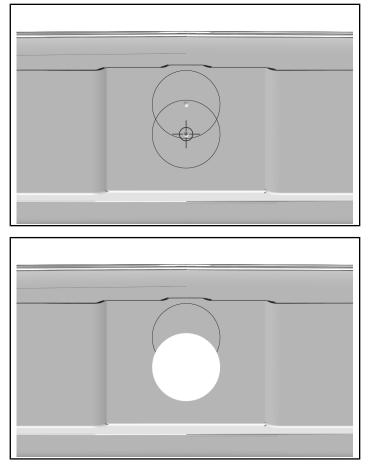
3. Connect the two sides of the circles. Cut remaining material inside the lines with a utility knife.
