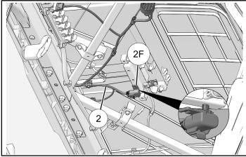
6. Install two kept rear roof screws. Torque screws to specification.
