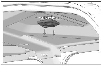
4. Crew Model Only: Remove five push dart clips from back of front roof liner.
