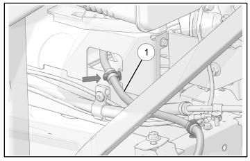
5. Attach up and down relays on box lift harness ① to rear seat mount bracket with two fir tree clips.
