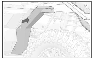
2. Attach rear wheel liner with three kept push-pin rivets.
