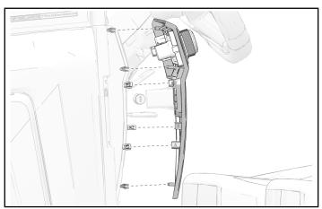
8. Install driver side trim panel to lower dash. Align tabs on top edge of the trim panel with dash opening and push into place.
