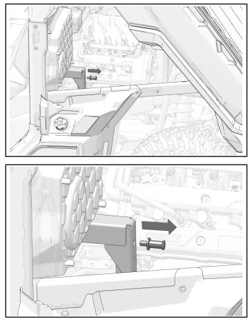
6. Install motor end of box lift actuator ② to chassis mounting bracket with kept clevis pin and hairpin clip.
