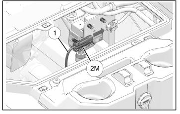
7. Install fir tree clip attached to connector **2M** on box lift harness ① to the rear seat mount bracket.
