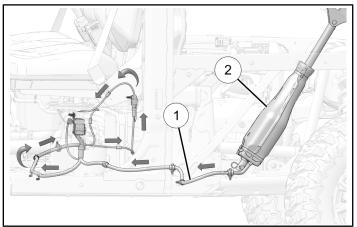
2. Connect **4F** on harness ① to box lift actuator ②.
