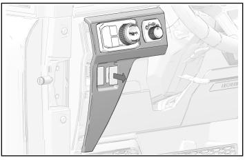
4. Put box lift switch ③ into opening on driver side trim panel. Push until it snaps into place.
