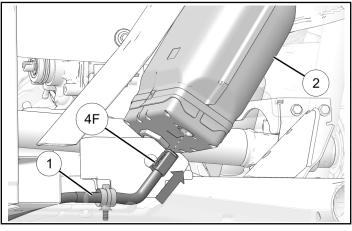
3. Attach lift box harness ① to rear lower chassis frame with three fir tree clips.
