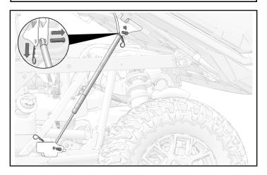
3. Remove strut. Strut and safety cable (if installed) will no longer be needed.
