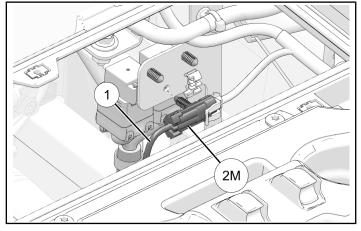
8. Route box lift harness ① toward passenger side of vehicle and attach to lower chassis frame with two standoff clips.
