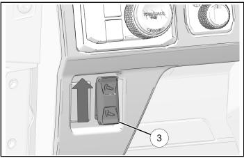
3. Push cargo box lift switch ③ down to lower cargo box.
