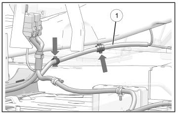
10. Install fir tree clip attached to box lift fuse **2F** to battery tray mount.
