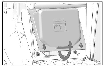
3. Disconnect negative cable first. Disconnect positive cable second.
