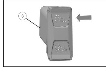
5. Connect box lift switch ③ to lift connector on chassis harness.
