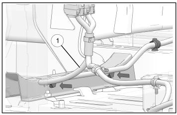
9. Route box lift harness ① toward battery and attach to lower chassis frame with two fir tree clips.
