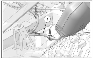
4. Attach box lift harness ① to rear seat mount bracket with one fir tree clip.
