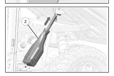
3. Install rod end of box lift actuator ② to bed mounting bracket with kept clevis pin and hairpin clip.
