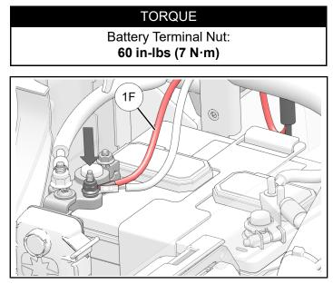
12. Attach negative terminal ring **1F** and negative battery cable to negative (-) connection on battery with kept nut.
