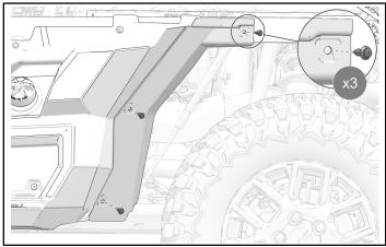
2. Remove driver side rear wheel liner and set aside.
