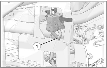
6. Connect box lift harness ① connector **2M** to chassis lift harness connector.
