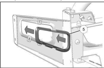
2. Install u-nuts ① on mounting tabs inside bumper.
