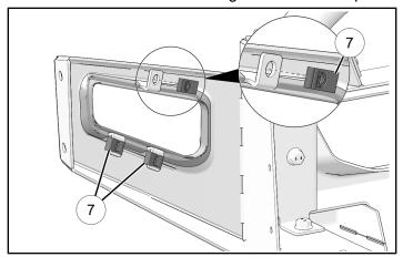
3. Install wiring harness ③. Attach to bumper using push pin clips and edge clips in positions show.
