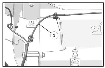
4. Route harness ③ along chassis tube. Attach using push pin clips and edge clips. Connect **2M** to chassis wiring harness.
