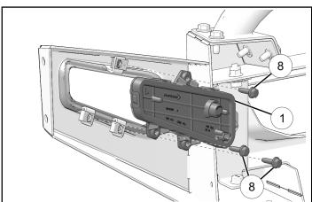
6. Connect wiring plug **3F** to light ①.
