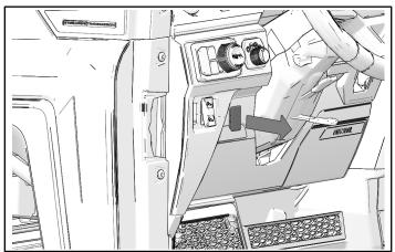
8. Remove panel. Use a pry tool to gently remove panel.
