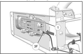
7. Remove blank switch plug in switch location shown.
