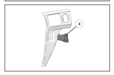
10. Pull wiring plug through opening and connect to switch 4.
