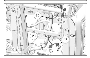
13. Install two fir tree clips into front close-off panel near **4F** connector on driver side.
