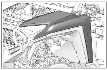
9. Install three screws into driver fender. Torque screws to specification.
