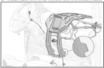
4. Attach upper center dash trim panel with four screws on top and two screws on lower edge of panel. Torque screws to specification.
