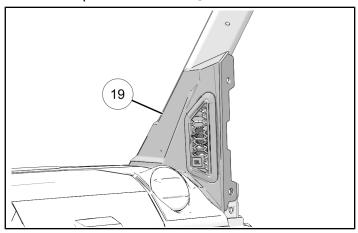
2. Connector tweeter ② connector to main audio harness connector **2F**.
