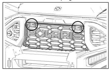
2. Remove two bottom grille tabs from vehicle while holding top tabs down.
