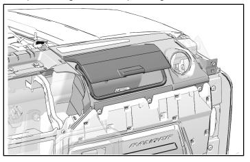
5. Remove one screw inside storage box, and three screws underneath storage box.
