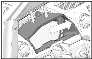
2. Remove four push-pin rivets from instrument bracket. Remove and disconnect instrument mount from vehicle.
