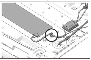
4. Install antenna receiver box into two shock mount panel holes.
