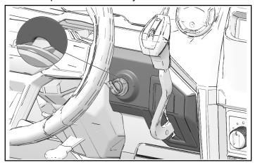
2. Install plastic nut around key. Install key if needed.
