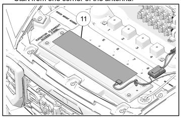
3. Install one fir tree clip on antenna harness into radiator cleanout access panel.
