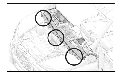
8. Install front driver fender onto vehicle.
