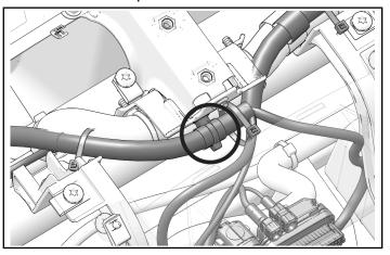
6. Remove cap from vehicle harness behind steering wheel.
