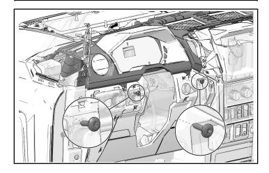
7. Install six screws into upper dash, two underneath passenger fender. Torque screws to specification.
