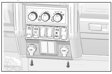
2. Turn control panel trim rearward and down to remove top two tabs from vehicle.
