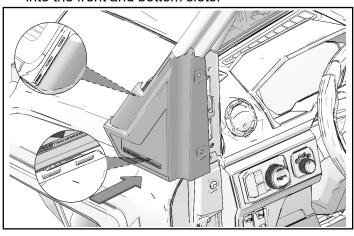
2. Install two push-pin rivets into a-pillar panel.
