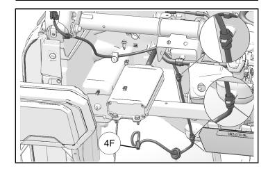
14. Pull both **4F** connectors through driver and passenger side storage holes. Make sure grommet is seated in holes.
