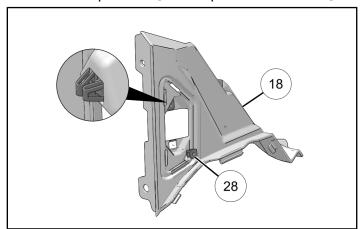
3. Install tweeter assembly ② into a-pillar audio cover with two screws ②. Torque screws to specification.
