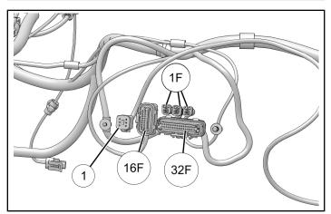
2. Install fir tree clip into support panel ① near the three **1F** connectors.
