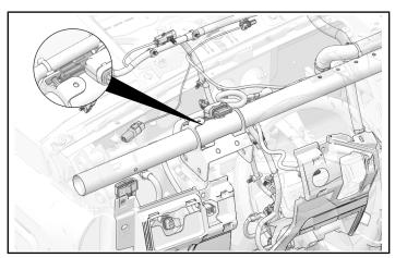
7. Connect connector 4M to vehicle harness.
