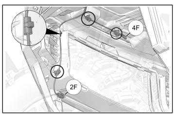
21. Install sensor gauge (9) near bottom of front fascia with fir tree clip. Connect sensor gauge (9) to connector **2F**.
