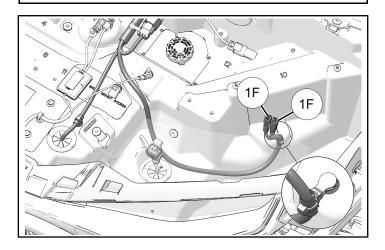
17. Install antenna (10) onto underhood liner with two screws (26). Torque screws to specification.
