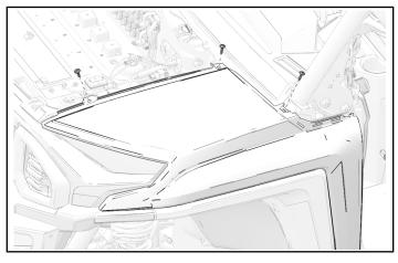
10. Install two screws in front of driver fender. Torque screws to specification.
