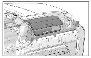
6. On driver side, install two screws from either side of the steering wheel. Torque screws to specification.
