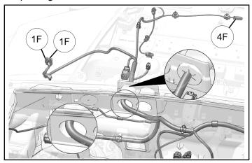
16. Route connectors **1F** underneath driver headlight. Attach connectors **1F** to underhood liner with edge clip.
