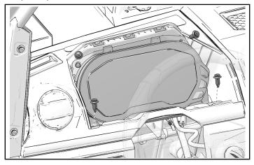
2. Install bottom clip of instrument bezel, then top clips.
