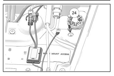
9. Install antenna terminal to stud using nut ②. Torque nut to specification.
