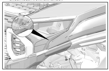
3. Remove two push pin rivets and four screws from under the fender.
