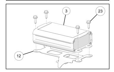
4. Move lower dash on driver side outward. Install bracket ② assembly with two screws ③ onto vehicle dash support to the left of the steering wheel. Torque screws to specification.
