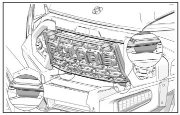
2. Install top two tabs into vehicle until it is seated.
