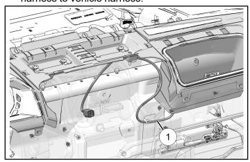
4. Install one screw inside storage box, and three screws underneath storage box. Torque screws to specification.
