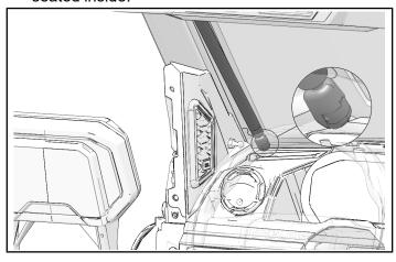
2. Install shock end onto ball end.
