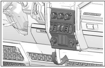
3. Attach with two push-pin rivets.
