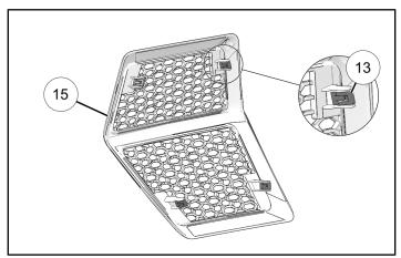
5. Install plastic speaker grille (5) onto front speaker. Make sure plastic clips (3) are installed into the four speaker slots.
