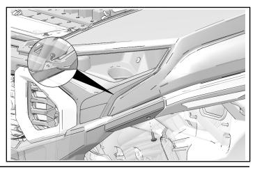
11. Install four screws into driver side cabin. Torque screws to specification.
