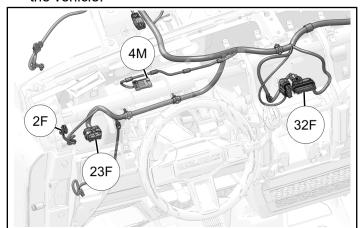
3. Install three cable ties ② on right side of ride command harness ⑥ to vehicle harness.
