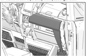
2. Remove trim clips from driver side. Disconnect any connections.
