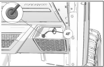
15. Route connectors **4F** and two **1F** through close-off panel grommet.
