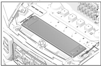
2. Remove adhesive backing from antenna (1) and attach antenna to radiator cleanout access panel. Start from one corner of the antenna.
