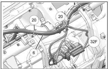
5. Install fir tree clip onto vehicle chassis.
