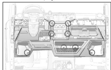
3. Install amp ③ onto bracket ⑫ using four screws③. Torque screws to specification.
