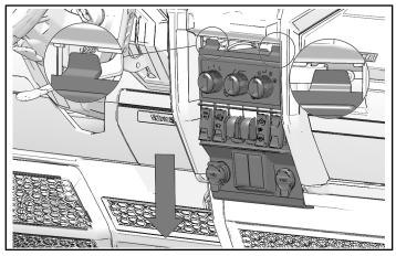
3. Remove center dash HVAC control panel trim and assembly. Disconnect any connections.
