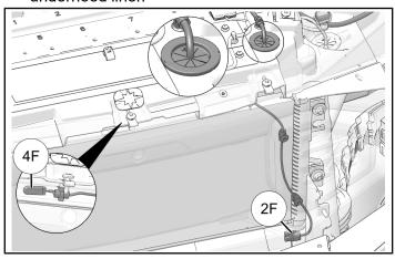
20. Attach four fir tree clips near connectors **4F** and **2F** onto front fascia and underhood liner.
