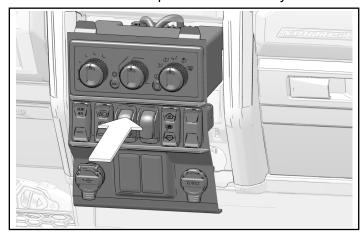
2. Move control panel trim up and forward to install two top tabs.
