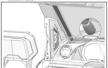
2. Install shock end onto ball end.
