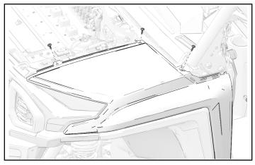
2. Remove six screws from upper dash. Screws will be under both front fenders.
