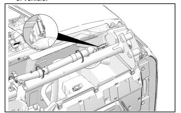
9. Connect connector **16M** to chassis harness. Install connector **16M** to vehicle beam using fir tree clip.
