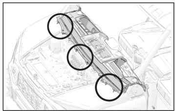
3. On driver side, remove two screws from either side of the steering wheel.
