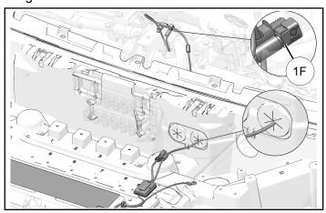
6. Attach antenna harness to vehicle harness with two cable ties ②.
