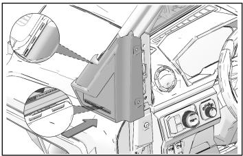
2. Install two push-pin rivets into a-pillar panel.
