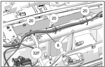
4. Install two cable ties ② near connector **32F** to vehicle harness
