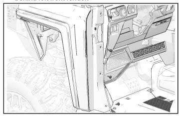
2. Remove and keep two screws near and underneath front left fender.
