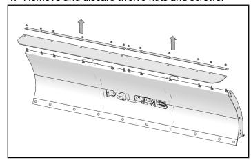
2. Remove and discard two flap brackets and flap.
