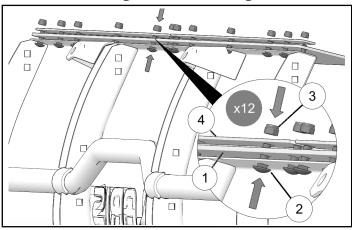
2. Tighten nuts ③ and screws ②starting at the center of each flap bracket ④ work outwards until all screws are seated evenly.
