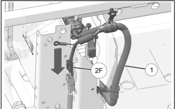
7. Install terminal ring **1F** on harness ① to charger bracket with kept charger bracket screw. Torque screw to specification.
