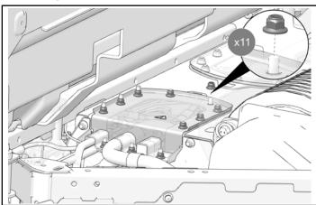
2. Remove and keep top panel from battery enclosure.
