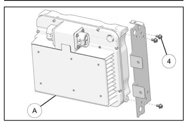
2. Attach front bracket to charger (A) with two screws(4). Torque to specification.
