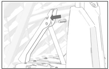
3. Install kept cotter pin through hole on clevis pin.
