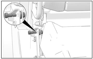
2. Remove and keep two bolts holding passenger seat to seat frame.
