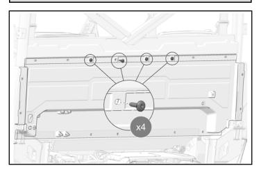
3. Attach top of rear close-off panel to vehicle with four kept push-pin rivets.
