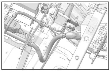
6. Remove terminal ring **1F** from ground connection near charge port.
