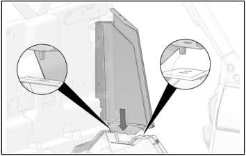
2. Attach upper side panel to rocker panel with one push-pin rivet.
