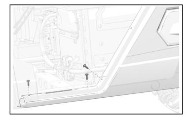
6. Attach upper door edge of rocker panel to vehicle frame with two kept push-pin rivets.
