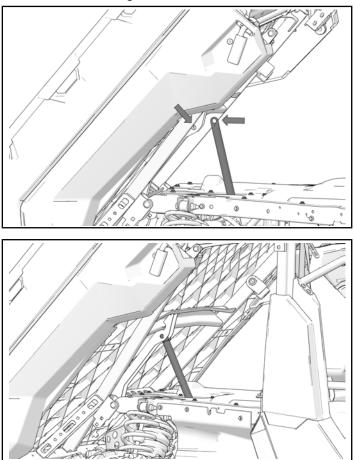
2. Attach shock to cargo box frame with kept clevis pin.
