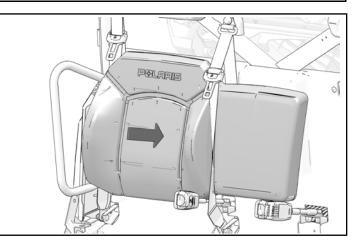
2. Attach passenger seat backrest to vehicle frame with four kept screws.
