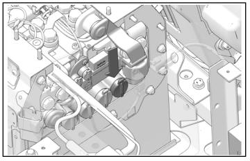
2. Remove and discard large plug from negative locations on the high voltage busbar.
