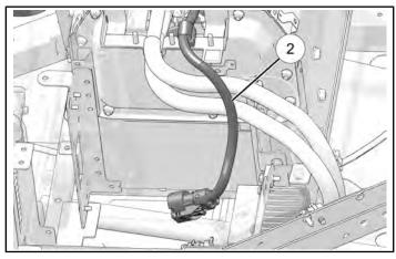
8. Align short harness ② with far right opening on top battery enclosure panel and install battery enclosure top panel onto studs.
