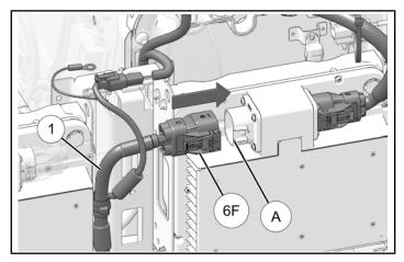
4. Install terminal ring **1F** on harness ① to charger bracket with kept charger bracket screw. Torque screw to specification.
