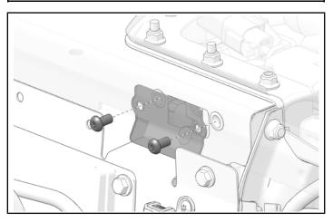
3. Torque screws to specification.
