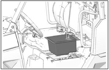
2. Install driver seat with seat slider onto the seat location in vehicle. Make sure that the front bracket fits into the holes of the bracket hinge.
