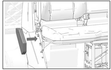
2. Attach seat pivot cover to seat frame with two kept screws.
