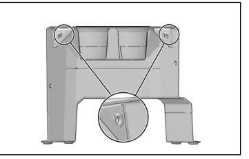
4. Remove tunnel cover from vehicle.
