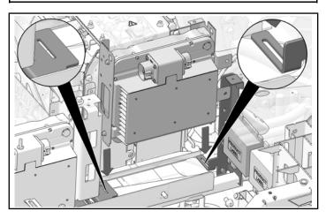
4. Attach rear charger bracket to chassis bracket with two kept bolts.
