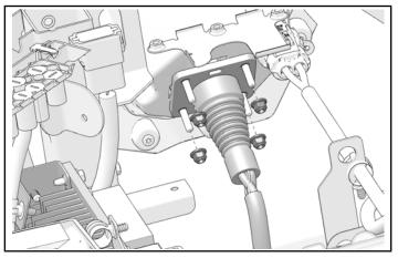
4. Torque nuts to specification.
