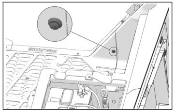
4. Remove and keep two screws from backside of floor panel.
