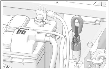
5. Connect the two-pin DC/DC connector (B), as shown.
