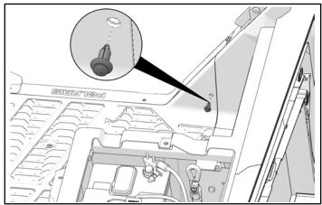
5. Attach floor panel to vehicle with eleven kept screws.
