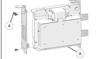
3. Align charger bracket ends with slots on existing chassis brackets.
