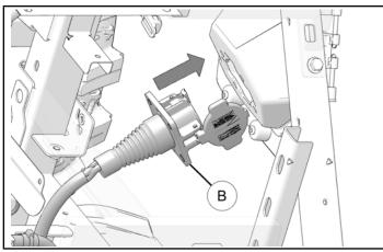
2. Attach charge port assembly to rocker panel with four kept screws.
