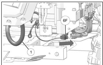
9. Install terminal ring **1F** on harness ① to port ground connection and attach with kept screw. Torque screw to specification.
