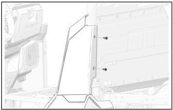
3. Remove and keep one upper side panel push-pin rivet.
