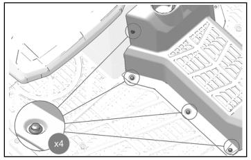
3. Install the left side with four kept push-pin rivets.
