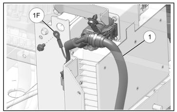
8. Install connector **6F** on harness ① to signal charge connection.
