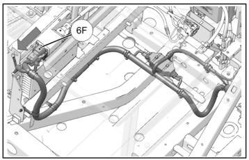
2. Remove and keep ground screw from front charger bracket.
