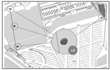
2. Remove and keep eleven screws from floor panel.
