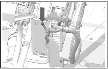
3. Remove terminal ring **1F** from ground connection on front charger bracket.
