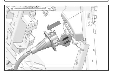
8. Remove rocker panel with charge port housing and set aside.
