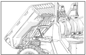
2. Remove and keep hairpin clip from shock attached to cargo box.
