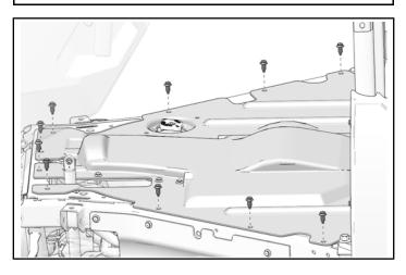
2. Remove and keep two screws from rear close-off panel.
