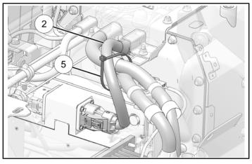
12. Install cable tie 5 around harness 1 and battery power cables.
