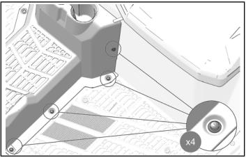
2. Remove and keep four push-pin rivets from tunnel cover.
