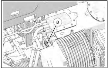
2. Connect high voltage test harness to the DC/DC connector on the vehicle.
