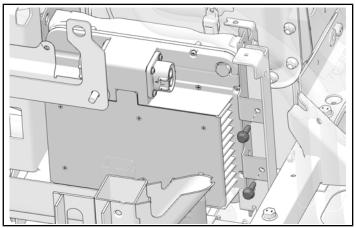
5. Torque charger bracket bolts to specification.
