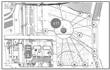
3. Remove and keep one push-pin rivet from side of floor panel.
