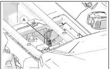
6. Slide the lock tab up, pinch the secondary lock, and then pull the plastic housing from the harness.
