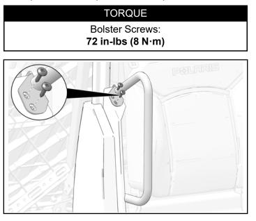
3. Attach bottom of bolster to seat frame with one bolt. Torque bolt to specification.
