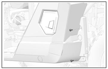
5. Pull side panel away from vehicle to access nuts. Remove and keep four nuts from charge port assembly.
