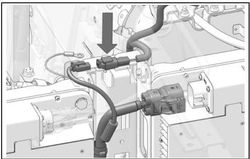
2. Install small connector **2F** on harness ① to chassis harness connector located on top of bracket.
