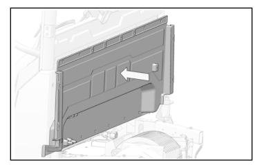
2. Attach top of rear close-off panel to vehicle with four kept screws.
