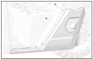
3. Remove and keep three screws from the door edge of the rocker panel.
