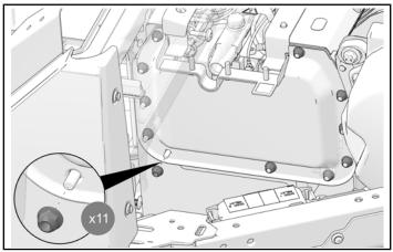
6. Torque nuts to specification.
