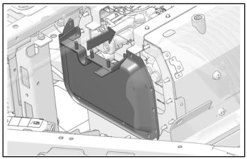
5. Attach side panel to battery enclosure with eleven kept nuts.
