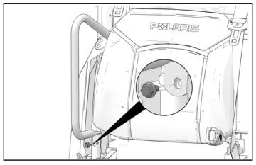
2. Remove and keep two upper bolster screws.
