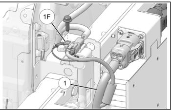
5. Connect harness plug **6F** on harness (1) to front connection on charger (B).
