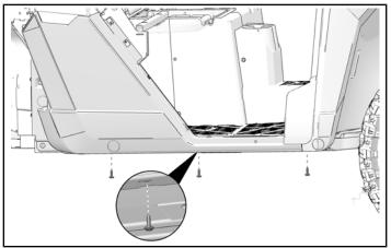
2. Remove and keep one push-pin rivet from door edge of the rocker panel.
