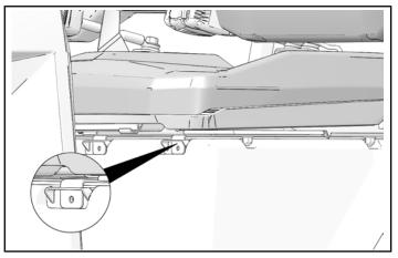
3. Install the two kept screws in front of the seat. Torque to specification.
