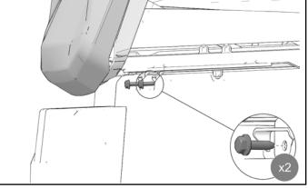
4. Move seat forward to install two kept underseat screws. Torque to specification.
