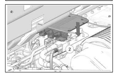
9. Attach top panel to battery enclosure with eleven kept nuts.
