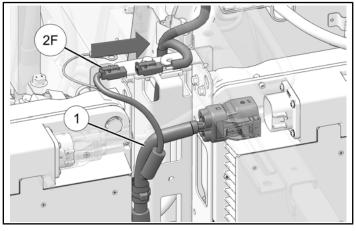
3. Connect harness plug **6F** on harness ① to front connection on charger (A).
