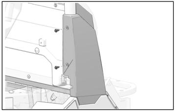
2. Remove and keep one push-pin rivet from lower side panel.
