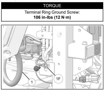
10. Attach harness ① to existing holes on chassis with push-pin darts.
