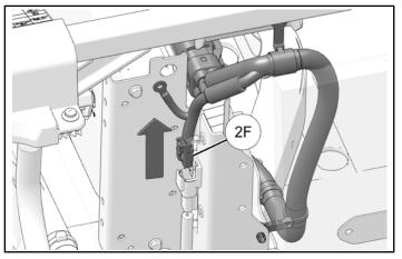
5. Remove and keep ground screw from bracket near charge port.
