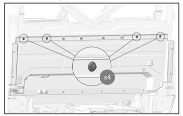
3. Remove and keep four screws from top of rear close-off panel.
