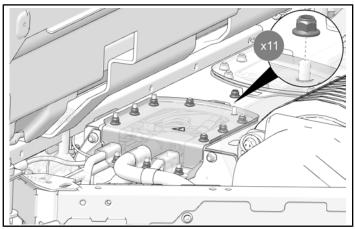
10. Torque nuts to specification.
