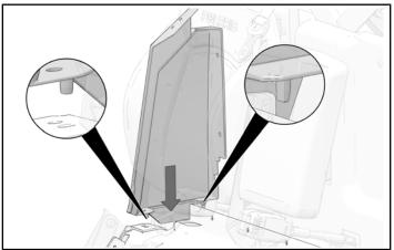
2. Attach upper side panel to rocker panel with one kept push-pin rivet.
