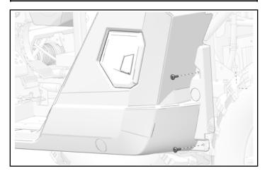
8. Attach bottom edge of rocker panel to vehicle frame with three kept screws.
