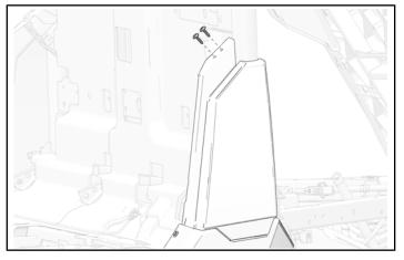
2. Remove and keep two push-pin rivets from upper side panel and rear close-off panel.
