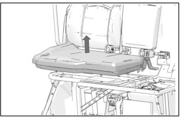
4. Remove and keep four screws holding seat backrest to vehicle frame.
