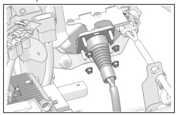
4. Torque nuts to specification.
