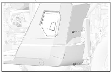
5. Pull side panel away from vehicle to access nuts. Remove and keep four nuts from charge port assembly.
