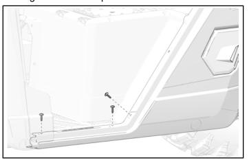
4. Remove and keep two screws from the rear edge of the rocker panel.
