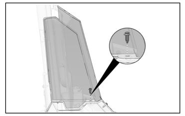
3. Attach upper side panel to vehicle frame and rear close-off panel with two push-pin rivets.
