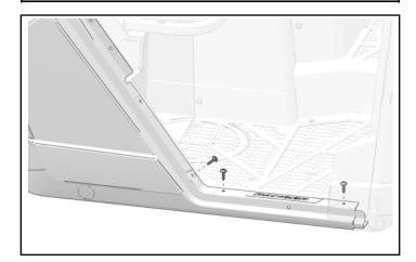
4. Attach upper door edge of rocker panel to vehicle frame with one kept push-pin rivets.
