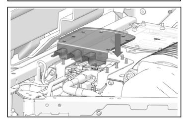
4. Attach top panel to battery enclosure with eleven nuts.
