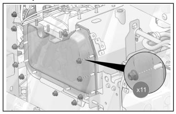
2. Remove and keep side panel from battery enclosure.
