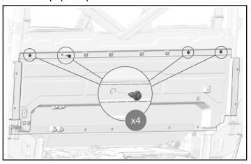
4. Attach bottom of rear close-off panel to vehicle with seven kept screws.
