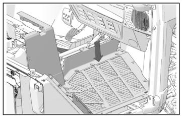
2. Attach floor panel to seat frame with two kept screws.
