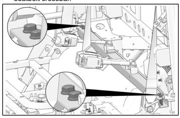
2. Move crossbar with seatbelts attached up over upper ROPS.
