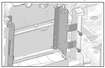
2. Remove and keep front charger mount bracket and one screw from in front of vehicle battery.
