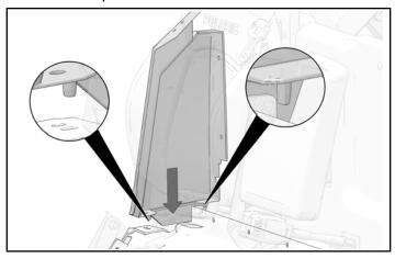
2. Attach upper side panel to rocker panel with one kept push-pin rivet.
