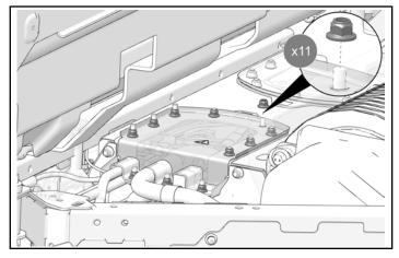
5. Torque nuts to specification.
