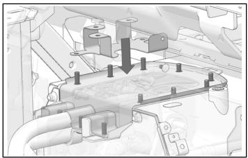
5. Attach top panel and bracket to battery enclosure with eleven nuts.
