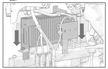
2. Attach converter and heat sink bracket to chassis bar with four kept bolts.
