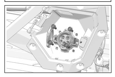
3. Attach charge port assembly to rocker panel with four kept nuts.
