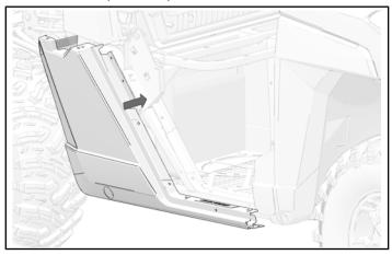
2. Attach rear edge of rocker panel to vehicle frame with two kept screws.
