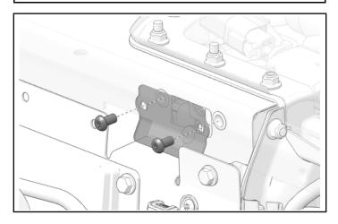
3. Torque screws to specification.
