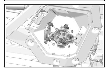
7. Remove charge port assembly and set off to the side. Charge port assembly will still be connected to the vehicle.
