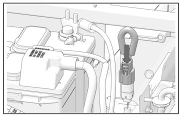
5. Connect the two-pin DC/DC connector  $\ensuremath{\mathbb{B}}$ , as shown.
