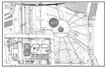
6. Torque screws to specification.
