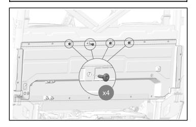
3. Attach top of rear close-off panel to vehicle with four kept push-pin rivets.
