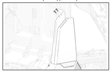
2. Remove and keep two push-pin rivets from upper side panel and rear close-off panel.
