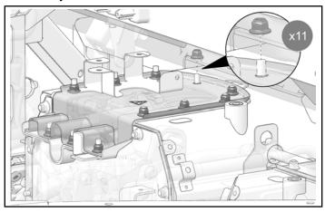
2. Remove and keep bracket from top panel of battery enclosure.
