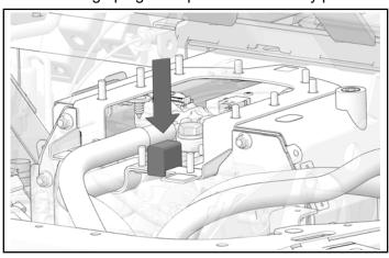
3. Install battery enclosure top panel onto studs.
