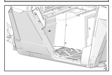
5. Attach bottom edge of rocker panel to vehicle frame with three kept screws.
