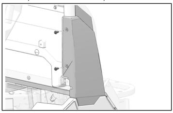
2. Remove and keep one push-pin rivet from lower side panel.
