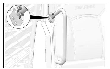
3. Attach bottom of bolster to seat frame with one bolt. Torque bolt to specification.
