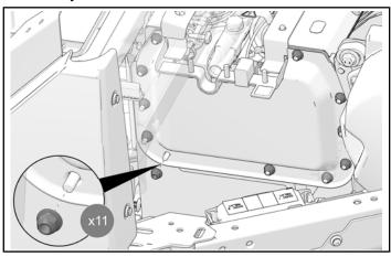
2. Remove and keep side panel from battery enclosure.
