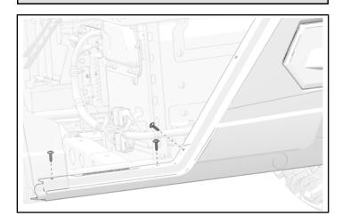
6. Attach upper door edge of rocker panel to vehicle frame with two kept push-pin rivets.
