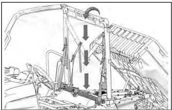
2. Align crossbar with fastener holes on vehicle frame.
