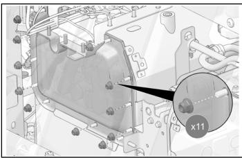
4. Torque nuts to specification.
