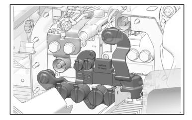
5. Attach ground wire and upper busbar to battery with screw (5).
