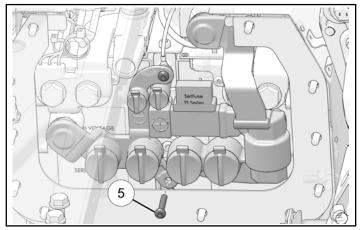
7. Torque screws 5 to specification.
