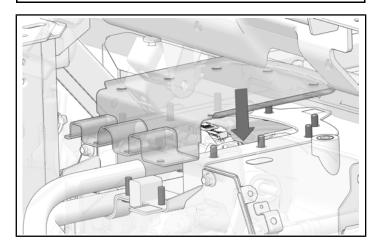
Install bracket onto battery enclosure top panel and studs.
