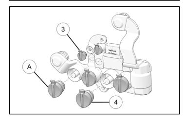
4. Install busbar onto battery connections.
