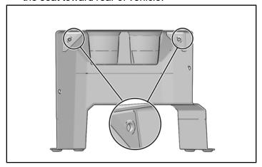
4. Remove tunnel cover from vehicle.
