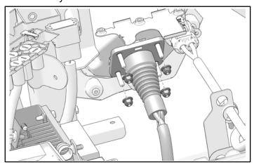
6. Open charge port cover. Remove and keep four screws from the charge port assembly.
