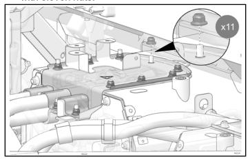
6. Torque nuts to specification.
