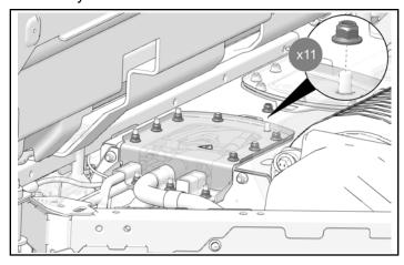
2. Remove and keep top panel from battery enclosure.
