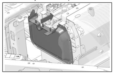
3. Attach side panel to battery enclosure with eleven nuts.
