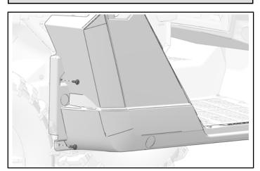
3. Attach door edge of rocker panel to vehicle frame with three kept screws.
