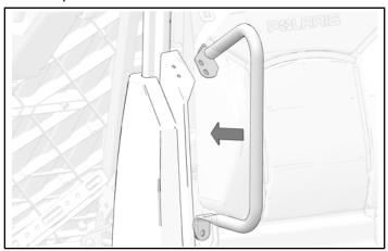
2. Attach top of bolster to upper side panel with two kept screws. Torque screws to specification.
