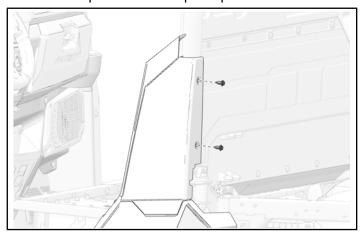
4. Attach upper side panel to vehicle frame bracket with two screws.
