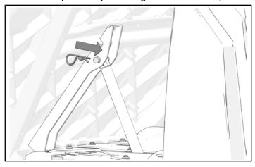
4. Lower cargo box and lock into position.
