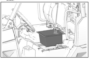
2. Install driver seat with seat slider onto the seat location in vehicle. Make sure that the front bracket fits into the holes of the bracket hinge.
