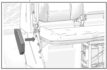
2. Attach seat pivot cover to seat frame with two kept screws.
