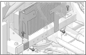
4. Move converter and heat sink away from the front battery enclosure panel.
