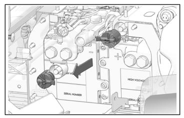
3. Install two existing plugs (A), two plugs (3), and two plugs (4) onto busbar.
