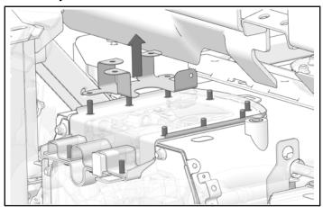
3. Remove and keep top panel from battery enclosure.
