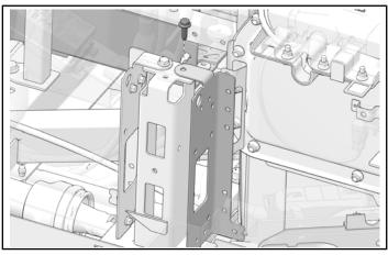
3. Torque screws to specification.
