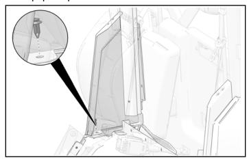
3. Attach upper side panel to vehicle frame and rear close-off panel with two kept push-pin rivets.
