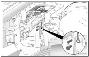
2. Remove and keep two plugs from battery.
