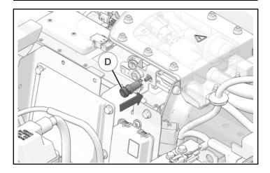
Install fuse cover onto each battery with two kept screws.
