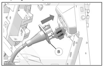
2. Attach charge port assembly to rocker panel with four kept screws.
