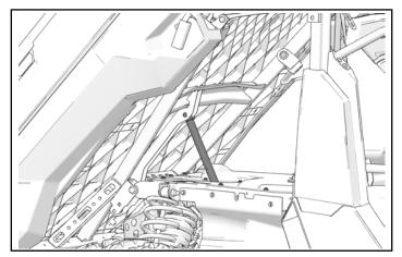
2. Attach shock to cargo box frame with kept clevis pin.
