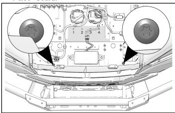
2. Remove and keep two screws at corners of bezel.
