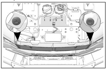
10. Install two screws at front of Polaris Pulse® board. Torque until fully seated.
