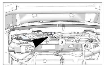
9. Install two screws at corners of bezel. Torque until fully seated.
