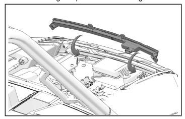
2. Install four screws (A). Torque until fully seated.
