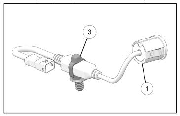
8. Clip bezel into place using four clips. Connect camera wiring to vehicle chassis harness. Make sure push pin clip ③ is secured.
