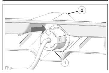
6. Install push pin clip ③ onto camera wiring ①.
