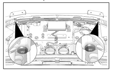
3. Lift up Polaris Pulse® board to access bezel clips. Push on four clips while gently pulling out on bezel.
