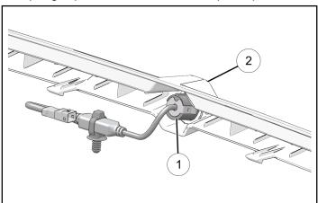
7. Install bezel assembly on vehicle. Guide camera wiring through opening to back side of grill. Make sure camera wiring does not get pinched.
