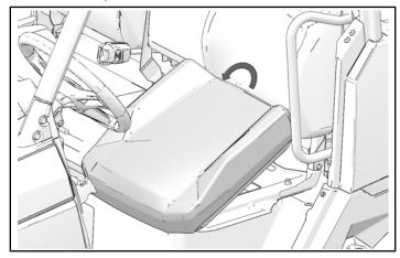
2. Slide seat forward to access underseat screws. Remove and keep two screws.
