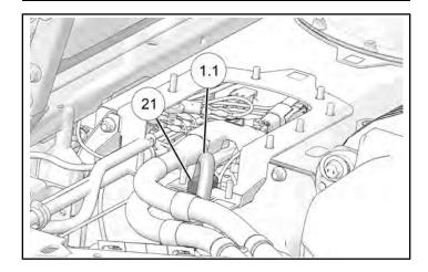
3. Install battery enclosure top panel onto studs.
