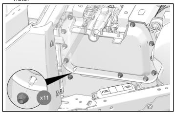
3. Torque nuts to specification.
