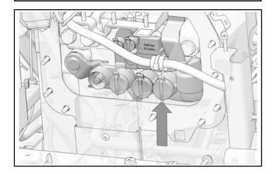
7. Install heater power harness 1.1 to busbar.
