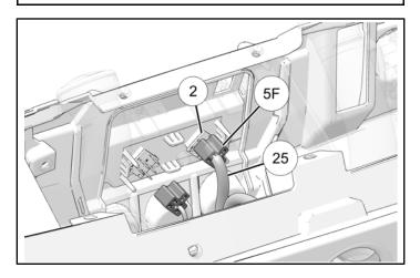
2. Connect temperature control connector **5F** on heater harness **(3)** to temperature connection on control panel **(2)**.
