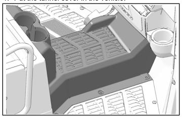
2. Install the right side with four kept push-pin rivets.
