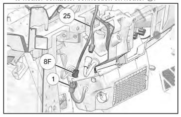
12. Install blower motor connector **4F**, on heater harness (3), to blower motor connection on heater
