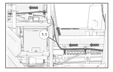
• Single battery heater power harness **1.1** routing:
