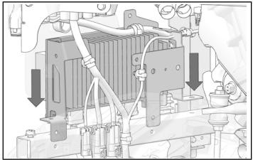
2. Install converter harness to chassis bar and converter brackets with five attached push-pin darts.
