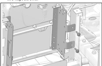
2. Attach front charger mount bracket to vehicle with one kept screw.
