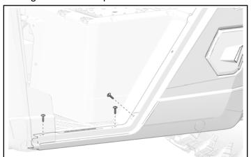
4. Remove and keep two screws from the rear edge of the rocker panel.
