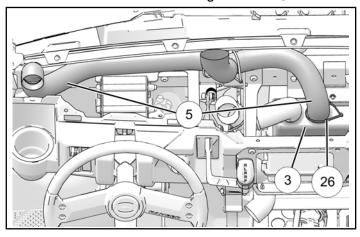
3. Install duct assembly ④ to far right outlet on manifold ③ until duct contacts stop on manifold. Attach duct to manifold using cable tie ⑥.
