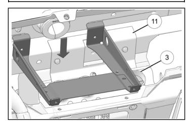
2. Attach dash support bracket to the chassis bar with two kept large screws.
