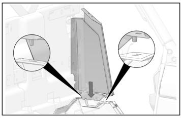
2. Attach upper side panel to rocker panel with one push-pin rivet.
