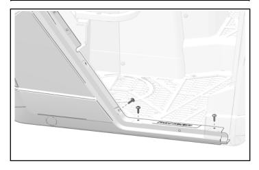
4. Attach upper door edge of rocker panel to vehicle frame with one kept push-pin rivets.
