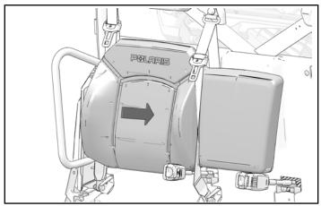
2. Attach passenger seat backrest to vehicle frame with four kept screws.
