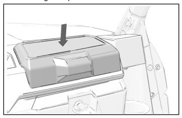
2. Install storage compartment to dashboard with four kept screws. Tighten until fully seated.
