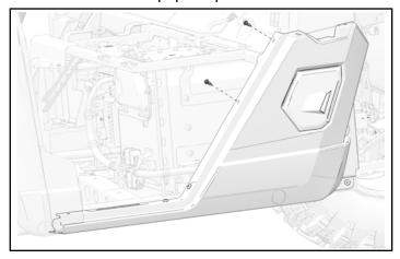
7. Attach rear edge of rocker panel to vehicle frame with two kept screws.
