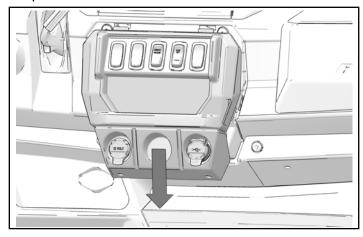
4. Label and disconnect electrical harnesses from switches, sockets, or other devices installed on control panel.
