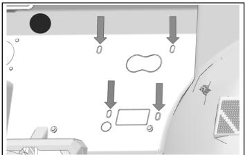
6. Drill one hole through embossed scribe line on the front close-off panel for drain nozzle on heater.
