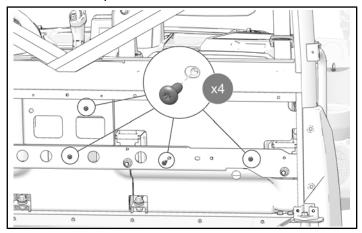
3. Torque screws to specification.
