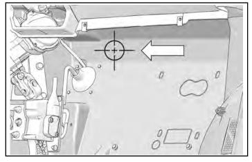
5. Drill two holes through each oval embossed scribe line on the front close-off panel for heater studs.
