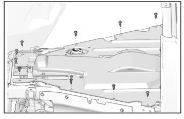
2. Remove and keep two screws from rear close-off panel.
