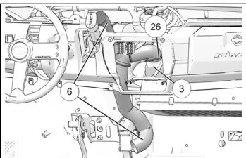
2. Install duct assembly ⑤ to center outlet on manifold ③ until duct contacts stop on manifold. Attach duct to manifold using cable tie ⑥.
