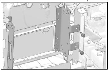
2. Remove and keep front charger mount bracket and one screw from in front of vehicle battery.
