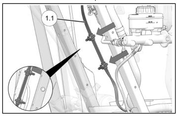
3. Route heater power harness **1.1** through vehicle tunnel toward rear of vehicle.
