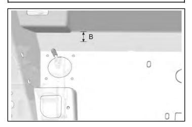
3. Drill pilot hole through front close-off panel for electrical harness.
