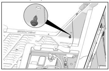
5. Attach floor panel to vehicle with eleven kept screws.
