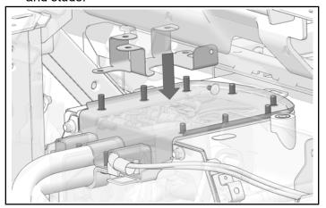
Attach top panel to battery enclosure with eleven nuts.
