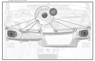
4. Attach lower dash to front close-off panel with four kept Hi/Lo screws.
