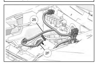
4. Remove terminal block cap on vehicle terminal block.
