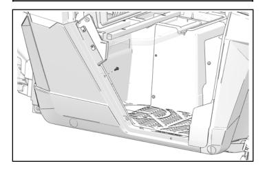
5. Attach bottom edge of rocker panel to vehicle frame with three kept screws.
