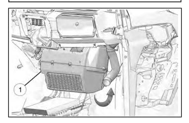
2. Slide heater studs and drain nozzle through drilled holes in front close-off panel.
