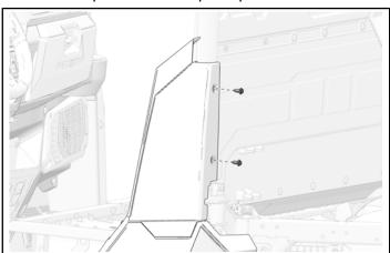
4. Attach upper side panel to vehicle frame bracket with two screws.
