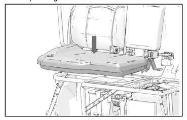
5. Attach passenger seat to seat frame with two kept bolts.
