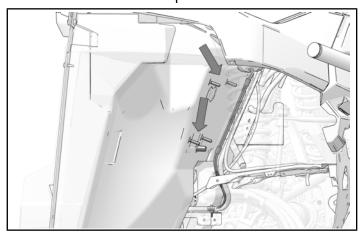
3. Loosely install heater ① to front close-off panel with four washers ② and four nuts ④.
