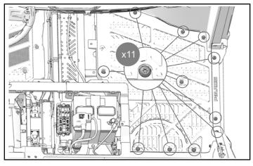
6. Torque screws to specification.
