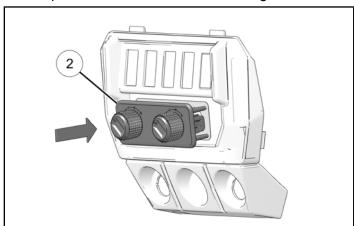
5. Push heater control panel ② into the control panel until the panel tabs lock in place.
