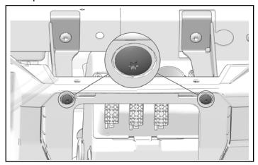
4. Tighten all four dash support bracket screws until fully seated.
