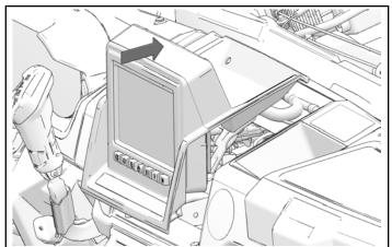
4. Attach Ride Command assembly to upper dash with two kept push-pin rivets.
