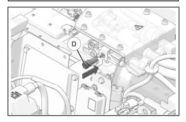
2. Install fuse cover onto each battery with two kept screws.
