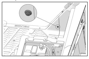
4. Remove and keep two screws from backside of floor panel.
