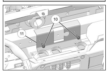
8. Loosely attach heater mounting bracket ① to heater with two nuts ②.
