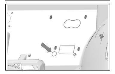
7. Cut out one round fresh air duct opening through embossed scribe line on the front close-off panel.
