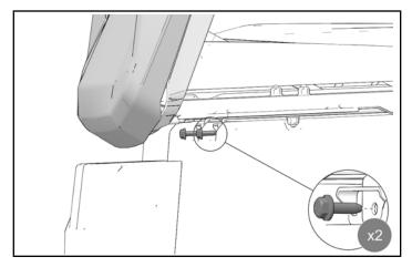
4. Move seat forward to install two kept underseat screws. Torque to specification.
