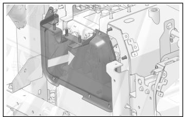
2. Attach side panel to battery enclosure with eleven
