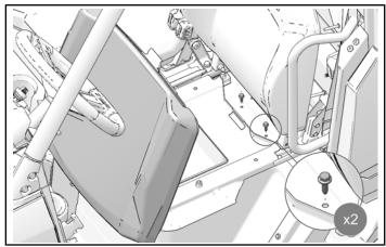
3. In front of the seat, locate two screws. Remove and keep two screws.
