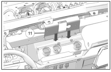
7. Loosely attach heater mounting bracket ① to front close-off panel with two screws ⑩.
