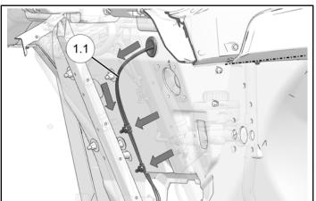
2. Attach heater power harness **1.1** to passenger side chassis bar with two push dart cable ties.
