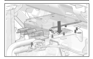
4. Install bracket onto battery enclosure top panel and studs.
