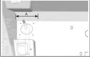
2. Measure down from top edge of face on the lower close-off panel to determine drill location. Mark this location.
