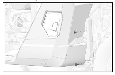
Pull side panel away from vehicle to access nuts. Remove and keep four nuts from charge port assembly.
