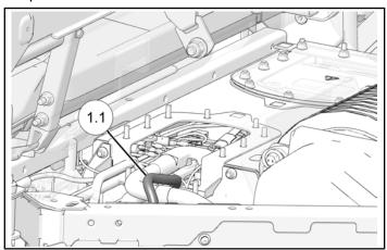
2. Install small plug ② into open slot under heater harness ①.
