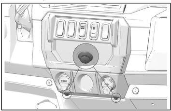
2. Pull bottom of control panel rearward to disengage two side tabs on the control panel from the main dash panel.
