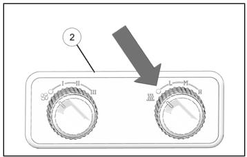
2. Use right side dial on heater control panel ② to control temperature settings.
