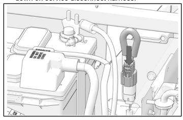
5. Connect the two-pin DC/DC connector  $\ensuremath{\mathbb{B}}$ , as shown.
