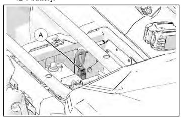
6. Slide the lock tab up, pinch the secondary lock, and then pull the plastic housing from the harness.
