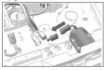
7. Install connector 6F to connected plug-in.
