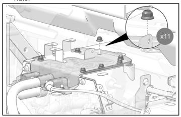
6. Torque nuts to specification.
