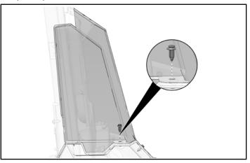
3. Attach upper side panel to vehicle frame and rear close-off panel with two push-pin rivets.
