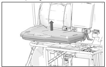
4. Remove and keep four screws holding seat backrest to vehicle frame.
