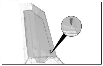
4. Lift upper side panel up and off of vehicle. Set upper side panel aside.
