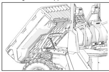
2. Remove and keep hairpin clip from shock attached to cargo box.
