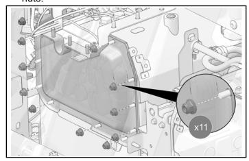
3. Torque nuts to specification.
