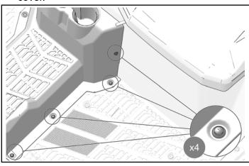
2. Remove and keep four push-pin rivets from tunnel cover.
