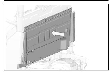
2. Attach top of rear close-off panel to vehicle with four kept screws.
