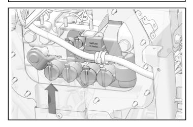
6. Remove and discard large plug on the positive (+) high voltage busbar.
