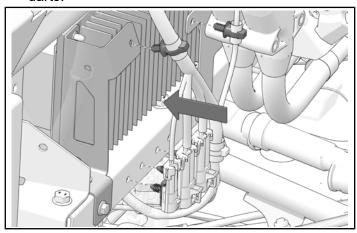
3. Attach converter and heat sink bracket to chassis bar with four bolts. Torque bolts to specification.
