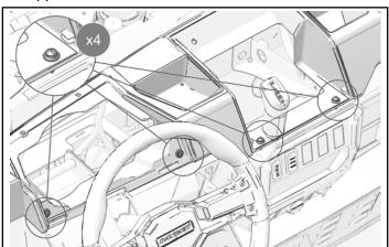
4. Install front of upper dashboard with six kept push-pin rivets.
