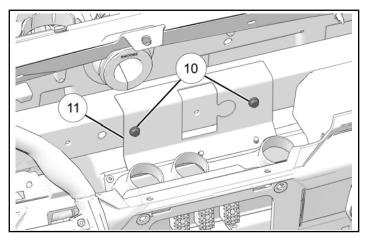
3. Torque heater mounting bracket nuts 1 to specification.
