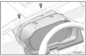
2. Remove the instrument cluster by pulling straight out towards the steering wheel.
