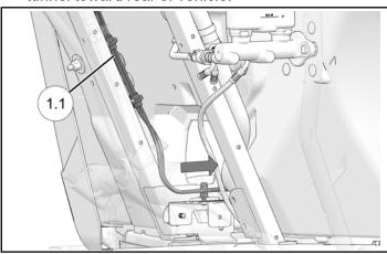
4. Route heater power harness **1.1** through vehicle tunnel toward rear of vehicle and to busbar connection on battery.
