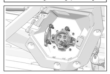
7. Remove charge port assembly and set off to the side. Charge port assembly will still be connected to the vehicle.
