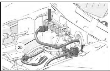
5. Install terminal block connector **3F** on the heater harness **(3)** to terminal block.
