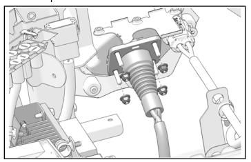
4. Torque nuts to specification.
