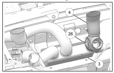
4. Install fresh air intake duct ⑦ to lower inlet on heater ① until duct contacts stop on heater inlet. Attach duct to manifold using cable tie 涵.
