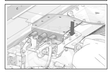
4. Attach top panel to battery enclosure with eleven
