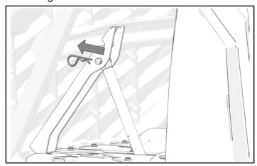
3. Remove and keep clevis pin from shock attached to cargo box.
