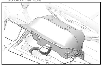
2. Install the instrument cluster bezel with two kept push-pin rivets.
