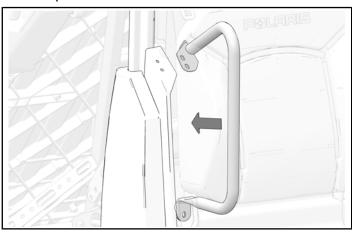
2. Attach top of bolster to upper side panel with two kept screws. Torque screws to specification.
