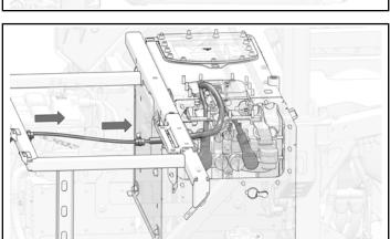
• Dual battery heater power harness 1.1 routing:
