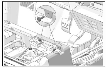
3. Torque screws to specification.
