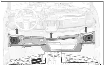
3. Attach lower dash to main dash with seven kept M6 screws.
