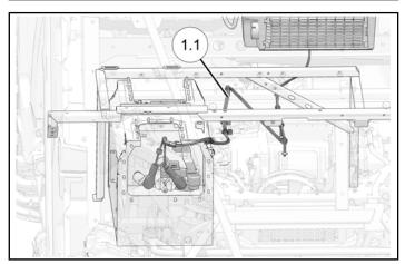
5. Remove and discard large plug on the negative (-) high voltage busbar.
