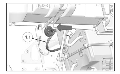
5. Route upper portion of right side dash duct assembly <sup>(3)</sup> into upper dash area.
