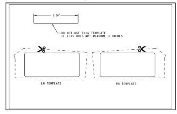
3. Tape each template to the underside of the upper dash, as shown.
