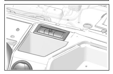
13. Move oval section of duct ⑤ to pre-cut dash opening.
