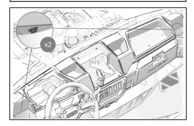
2. Install two kept push-pin rivets on passenger's side of upper dashboard.
