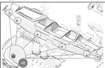
2. Remove and keep four push-pin rivets from driver's side of upper dashboard.
