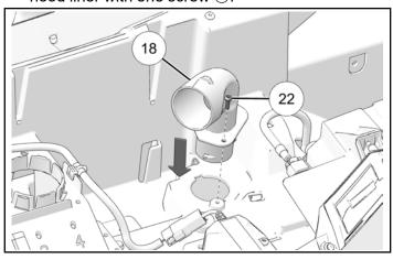
2. Torque screw to specification.
