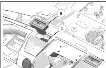
15. Push vent and duct down into upper dash opening until vent locks into place on upper dash.
