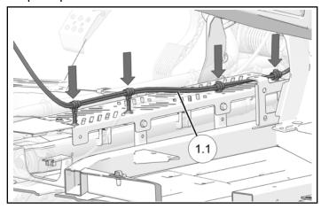
2. Attach heater power harness 1.1 to brackets with pre-installed edge clips.
