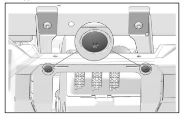
3. Remove and keep two screws from dash support bracket and the chassis.
