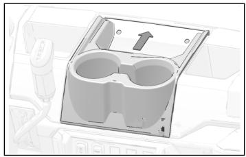
2. Install cup holder with two kept push-pin rivets.
