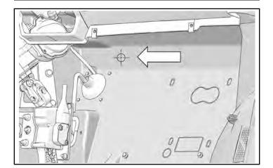
4. Drill larger hole through pilot hole on the front close-off panel for heater harness grommet.
