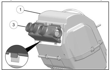
5. Attach the manifold ③ to the heater ① with two screws ⑨.
