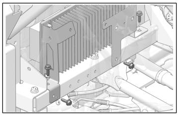
4. Move converter and heat sink away from battery enclosure panel side panel.
