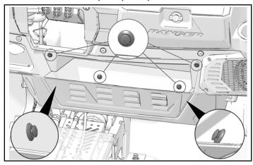
2. Remove storage bin. Storage bin will not be reinstalled.
