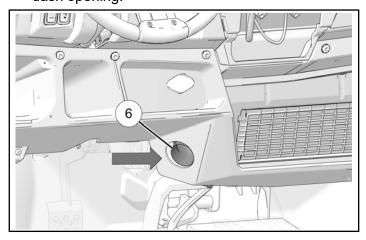
4. Install vent ① onto duct ⑥. Attach vent to duct with cable tie ⑥.
