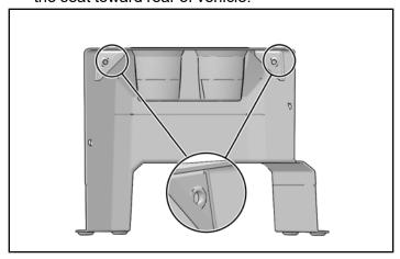
4. Remove tunnel cover from vehicle.
