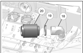
5. Torque clamp screw to specification.
