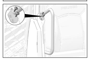
3. Attach bottom of bolster to seat frame with one bolt. Torque bolt to specification.
