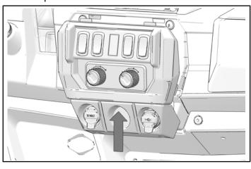
5. Install two side tabs on control panel to main dash panel.
