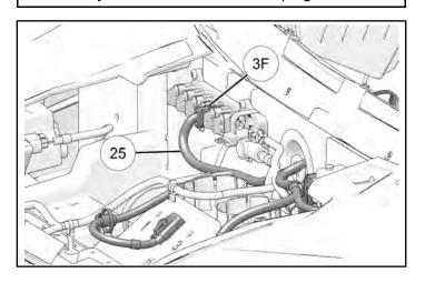
6. Disconnect chassis harness from connected plug-in.
