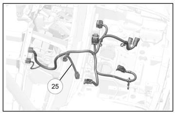
2. Route blower control connector **5F**, heater control connector **5F**, heater connector **8F**, and blower motor connector **4F**, on heater harness **(35)**, through grommet into upper dash area. All remaining heater connections will be installed in under hood area.
