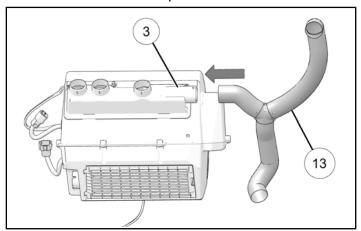
2. Attach right dash duct assembly <sup>®</sup> to manifold <sup>®</sup> with cable tie <sup>®</sup>.
