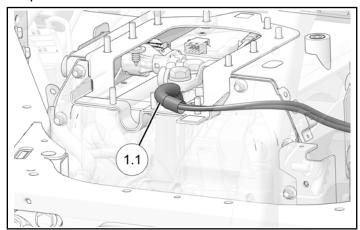
2. Install small plug ② into open slot with heater harness 1.
