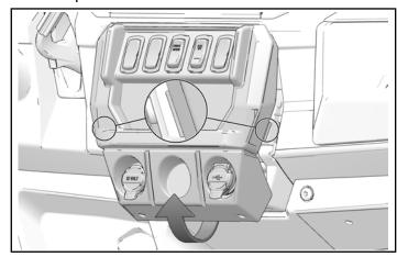
3. Pull control panel down to disengage two upper tabs on the control panel from the main dash panel.
