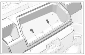
3. Install four kept push-pin rivets on driver's side of upper dashboard.
