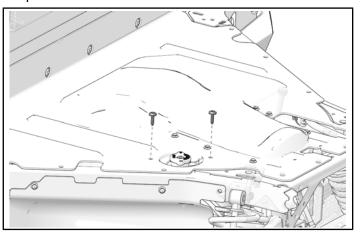
3. Carefully lift up close-off panel and disconnect fan.
