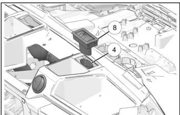
12. Push vent and duct down into upper dash opening until vent locks into place on upper dash.
