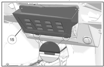
2. Attach lower storage compartment (5) to lower dash panel with two kept push-pin rivets.
