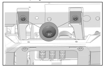
3. Attach dash support bracket to the dash with two kept small screws.
