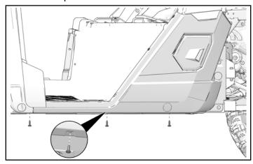
2. Remove and keep two push-pin rivets from door edge of the rocker panel.
