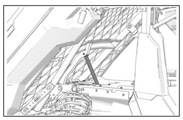
3. Install kept cotter pin through hole on clevis pin.
