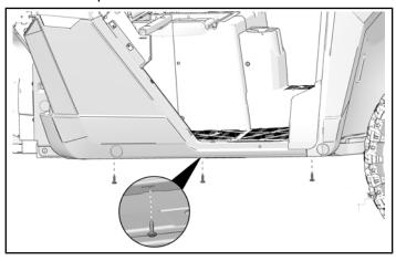
2. Remove and keep one push-pin rivet from door edge of the rocker panel.
