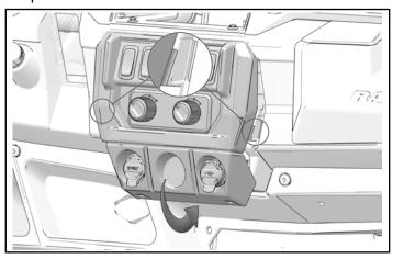
6. Attach control panel to upper dash with two kept push-pin rivets.
