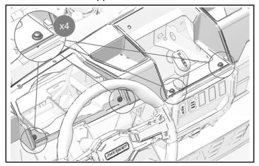
3. Remove and keep two push-pin rivets from passenger's side of upper dashboard.
