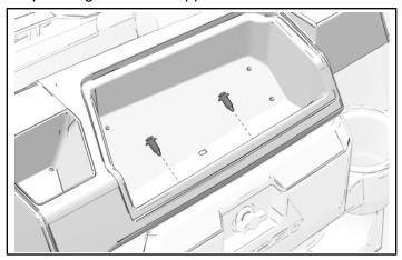
4. Remove and keep two push-pin rivets from underside of upper dashboard.
