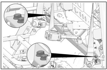
2. Move crossbar with seatbelts attached up over upper ROPS.
