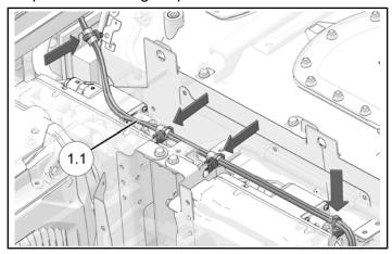
3. Attach edge clips on heater power harness 1.1 to brackets with cable ties 26.
