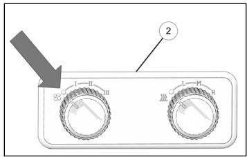
2. Use left side dial on heater control panel ② to change fan speed.
