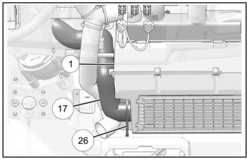
5. Move fresh air duct ① up and through pre-cut opening in the front close-off panel.
