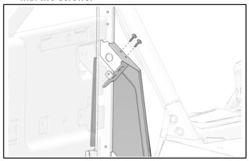
5. Torque screws to specification.
