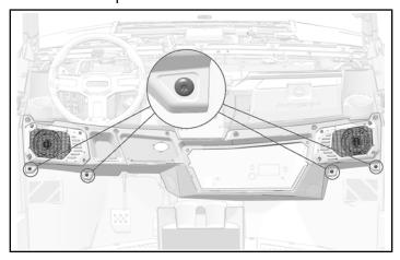
3. Remove and keep seven screws from lower dash panel.
