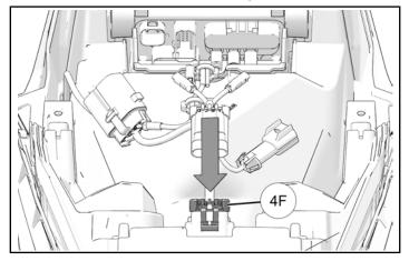
5. Attach connector **4M** to existing headlight connection on snowmobile.
