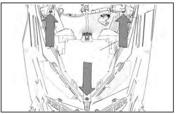
4. Pull headlight assembly back and up to remove from hood.
