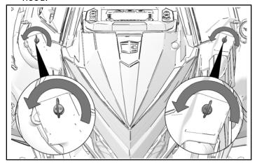
2. Pull sides of hood out away from side panel fasteners.
