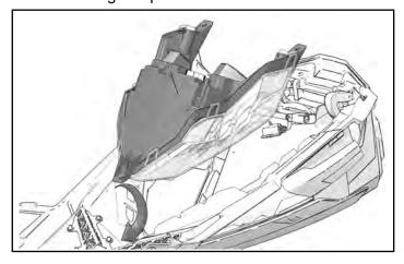
2. Attach headlight using four screws.
