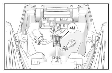
6. Connect two 2M connectors to auxiliary lights.
