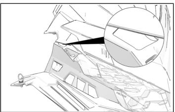
6. Attach auxiliary light using tool (6) (not shown) and two screws (4) (not shown) in positions shown. Use existing hole and drilled hole. Torque screws until fully-seated.
