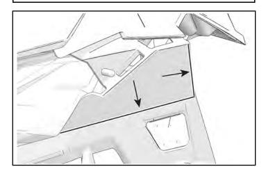
4. Use supplied template located on box flap to mark drill location. Drill hole on mark.
