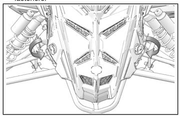
3. Turn hood fasteners clockwise to lock hood.
