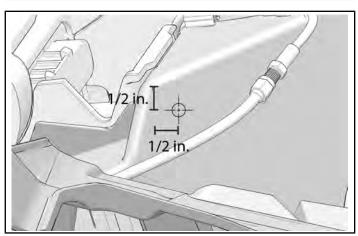
2. Locate connector **8F** and attached push pin clip on wiring harness ①
