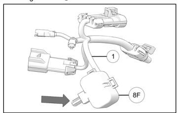
3. Attach wiring harness in drilled hole using push pin clip on connector **8F**.
