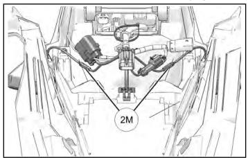
7. Remove tape and protective cap from existing power connection on snowmobile. Keep protective cap.
