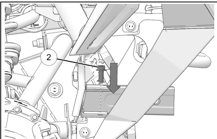
4. Loosely install two screws ② in upper holes of receiver.
