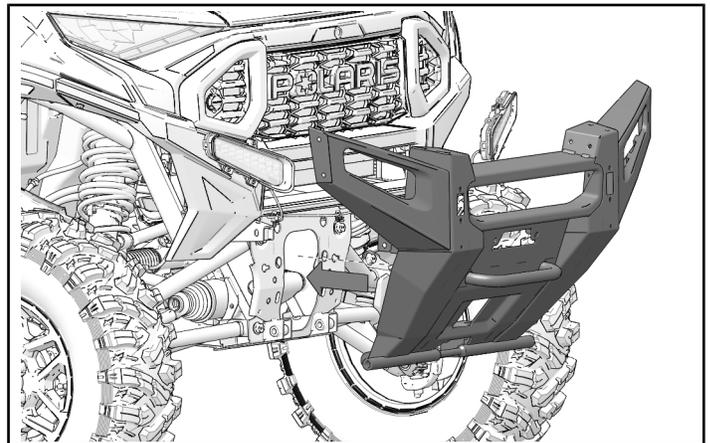
2. Support weight of bumper while installing screws. Install four screws. After all four screws are installed, torque screws to specification.
