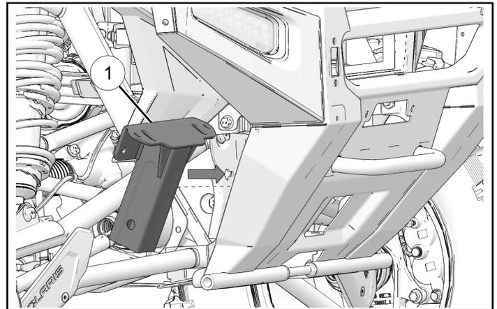
2. Rotate receiver into proper position through front bumper hole.
