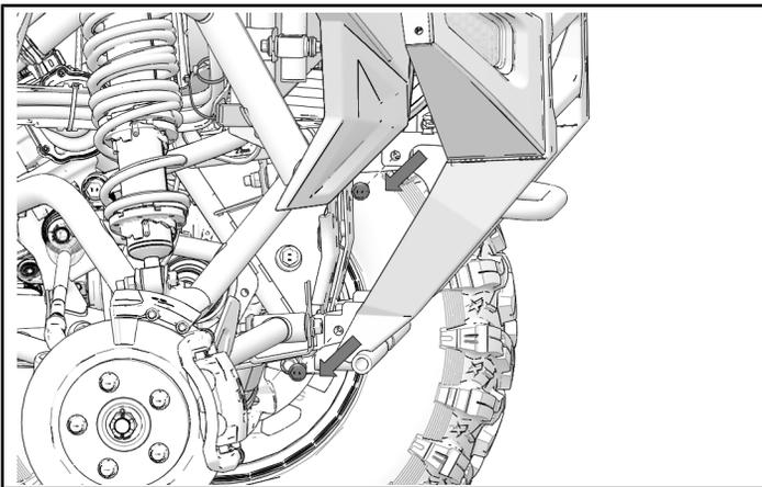
2. Pull forward to remove front bumper from vehicle.
