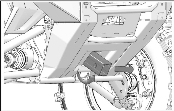
3. Loosely install two screws ② in lower holes of receiver.
