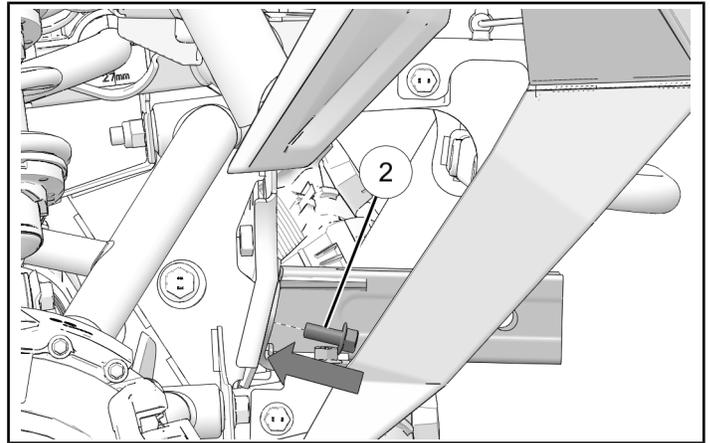
5. Tighten four screws ② to specification.
