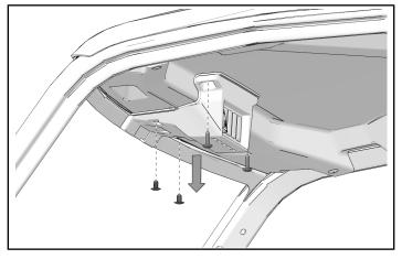
2. Disconnect wire harnesses from back of switches. Remove and keep switch panel.
