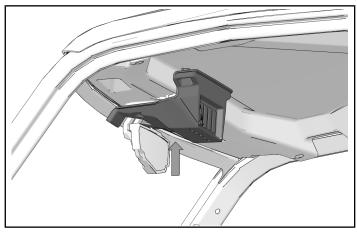
2. Install two push darts and two screws. Torque screws to specification.
