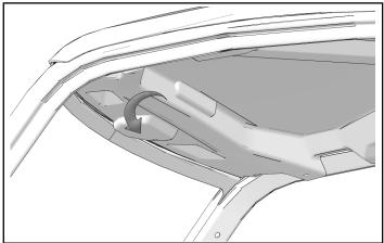
3. Locate rear view mirror trim line on top surface of roof liner. Cut along line to trim roof liner.
