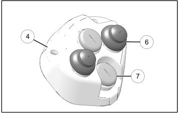
4. Install shifter handle harness ® along bottom of plow handle ③ and connect to plow control switches ⑥ or caps ⑦.
