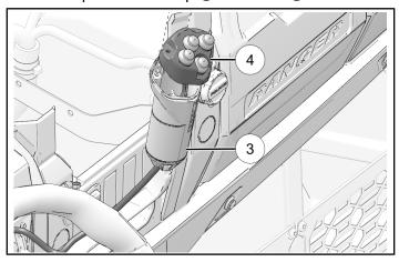
7. Attach plow control top 4 to handle with screws5. Tighten screws until fully seated.
