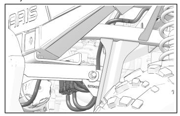
6. Install left and right relays to winch mount with push-darts ①. Install tilt circuit breaker to winch mount with attached push-dart.
