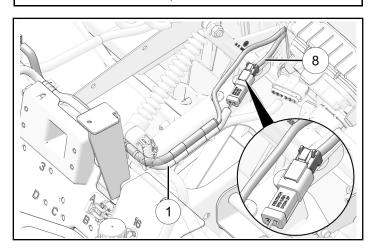
10. Remove cap from winch splitter connector and connect plow control harness ① to shift handle harness ⑧.
