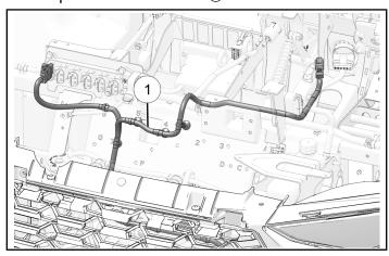
2. Remove plug from Polaris Pulse® bar and install power connector.
