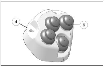
• For angle control only, install two switches ⑥ into plow control top. Close top and bottom holes with caps ⑦.
