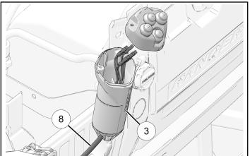
5. Attach harness with three zip ties, one under handle, one half way down handle, and one before harness exits bottom of handle.
