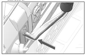
9. Connect shifter handle harness to plow control harness.
