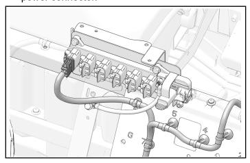
3. Install harness along electrical mount as shown using, attached push-darts.
