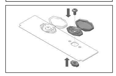
2. Slide assembled bracket and fastener assemblies into desired position on rack. When bracket is in desired position, torque screws to specification.
