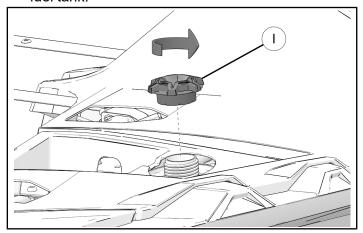
13. Remove fastener M under deck hump.
