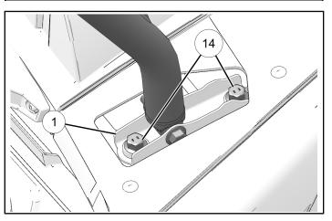
8. Loosely install cap screws ① to secure front of frame ③.
