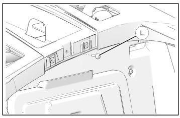
16. Remove two screws @ from rear of deck.
