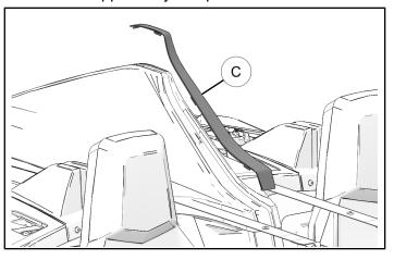
4. Remove trim piece at rear of upper body. If equipped with rear back-up camera, disconnect electrical connector.
