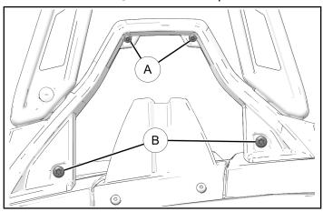
3. Remove and keep two fasteners © on back of hoop trim.
