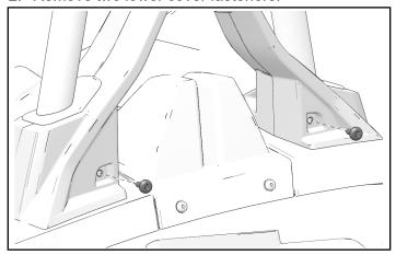
3. Remove two rear cover fasteners.
