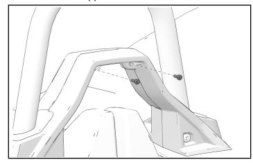
2. Remove two lower cover fasteners.
