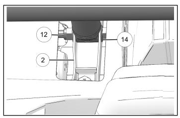
7. Loosely install screws (4) to secure outer frame mounts to the vehicle.
