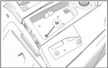
9. Install trim piece at rear of deck. If equipped with back-up camera, install camera assembly.
