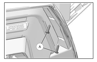
2. Remove two push pin rivets ® from underside of trim piece.
