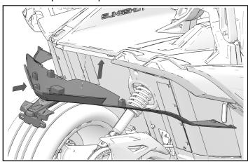
2. Install seven retained fasteners (A) and two retained fasteners (B) to rear lower cover. Torque fasteners to specification.
