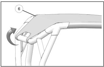
5. Slide semi-rigid front edge of top out of the mounting channel at front of frame assembly.
