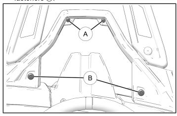
3. Remove two fasteners © on back of hoop trim.
