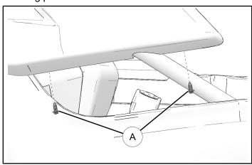
2. Remove and keep two fasteners (B) under wing panel.
