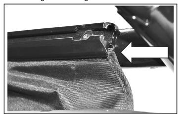
4. Route the top over the front of the frame assembly and unroll toward the rear of the vehicle. Make sure the top remains evenly spaced on the frame assembly.
