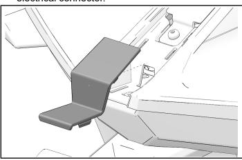
5. Remove and keep upper body trim fasteners (D) and lift trim piece (E) away from vehicle. If equipped with center tail lamp, disconnect electrical connector.
