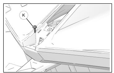
4. Install screw ① located behind seat headrest.
