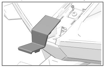
10. Install upper body trim (E) and secure with fasteners (D). Connect wiring if equipped with center tail lamp.
