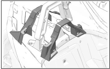
5. Remove two fasteners ① from deck hump.
