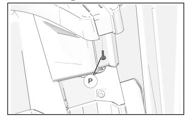
18. Pull out on side wings and lift rear deck away from vehicle.
