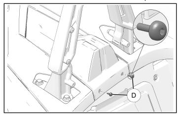
6. Lift front edge of deck hump and pull forward to remove.
