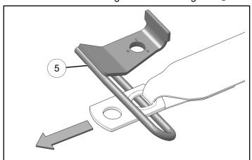
2. Install seat belt. Make sure seat belt mount washer is centered on bolt shoulder and seat belt mount pivots freely around mounting bolt.
