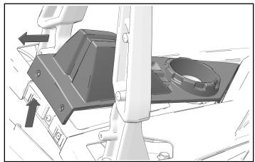
9. Install fuel cap to make sure debris does not fall into tank during vehicle service.
