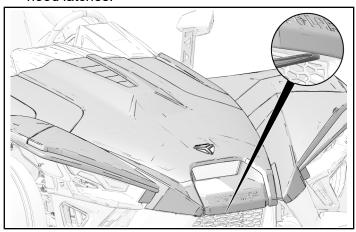
3. Pull upwards on hood underside, above LED lamp, using two hands.
