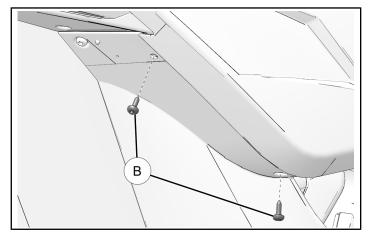
7. Install two push pin rivets (A) under wing panel.
