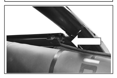
3. Slide the semi-rigid front edge into the channel. Make sure the top is centered in the channel by matching the overhang amount on each side.
