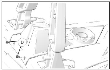
8. Lift front edge deck hump and pull forward to remove.
