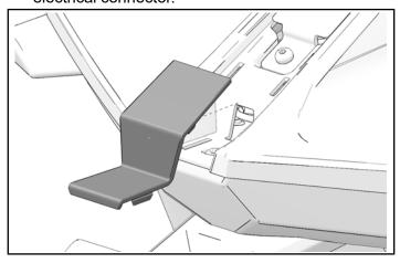
8. Remove and keep upper body trim fasteners ① and lift trim piece ⑥ away from vehicle. If equipped with center tail lamp, disconnect electrical connector.
