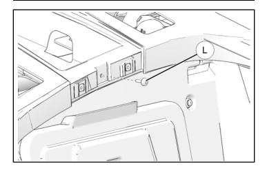
11. Remove two screws @ from rear of deck.
