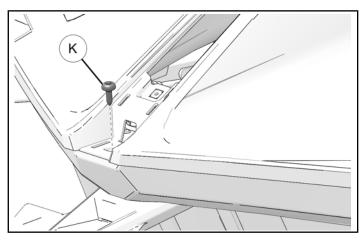
4. Install screw (1) located behind seat headrest.
