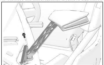
2. Remove two mounting plate fasteners and mounting plate from vehicle.
