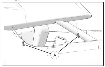
4. Remove and keep two fasteners (B) under wing panel.
