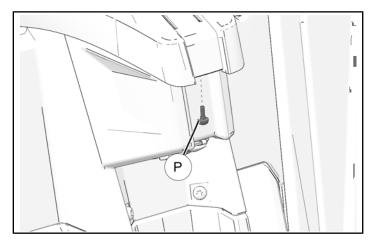
6. Install two fasteners ® under wing panel.
