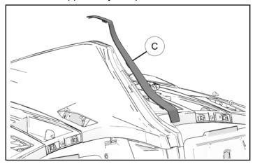
7. Remove trim piece at rear of upper body. If equipped with rear back-up camera, disconnect electrical connector.
