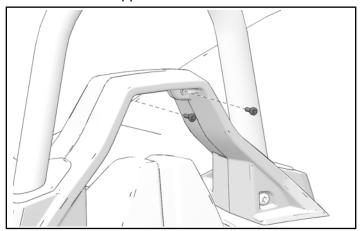
2. Remove two lower cover fasteners.
