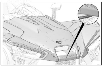
3. Pull upwards on hood underside, above LED lamp, using two hands.
