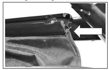
Route the top over the front of the frame assembly and unroll toward the rear of the vehicle. Make sure the top remains evenly spaced on the frame assembly.
