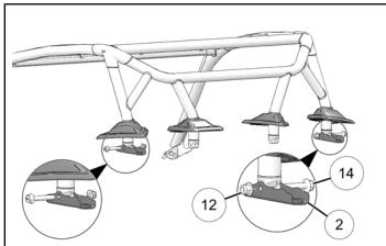
4. Install frame assembly ③ on vehicle. Make sure frame is placed on inner mounts ① and ②.
