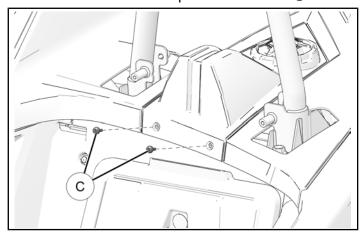
3. Pull deck hump ① forward slightly the lift front of deck up to remove from vehicle.
