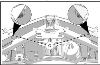
12. Pull out on side wings and lift rear deck away from vehicle.
