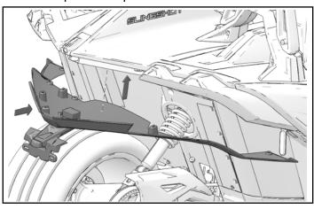
2. Install seven retained fasteners (A) and two retained fasteners (B) to rear lower cover. Torque fasteners to specification.
