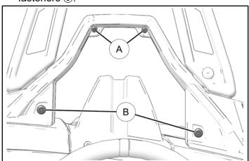
3. Remove two fasteners c on back of hoop trim.
