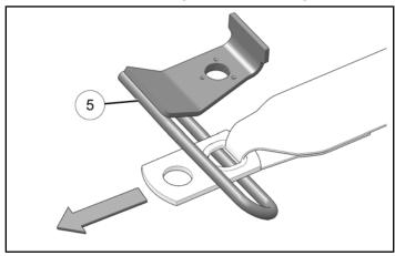
Install seat belt. Make sure seat belt mount washer is centered on bolt shoulder and seat belt mount pivots freely around mounting bolt.
