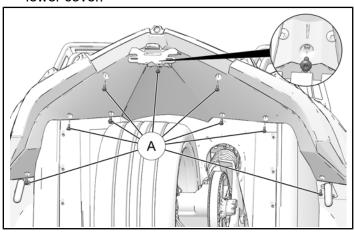
2. Lower panel from vehicle and disconnect any electrical connectors. Carefully set aside panel.
