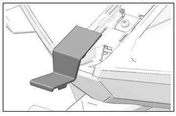
10. Install upper body trim (E) and secure with fasteners (D). Connect wiring if equipped with center tail lamp.
