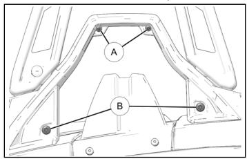
3. Remove and keep two fasteners c on back of hoop trim.
