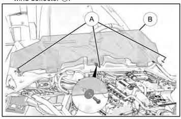
2. If equipped, remove and keep screw, washer and O-ring from center wind deflector mount.
