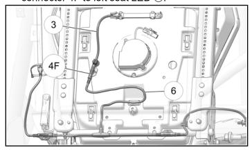
4. Attach left rear interglow harness extension **6** to seat using clips **b** and **b**.
