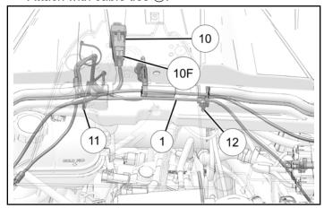
3. Route multicolor interior LED harness ① along existing harness. Put through firewall along existing wiring. Connect plug 2F to chassis harness 2M. Attach with cable ties ⑪.
