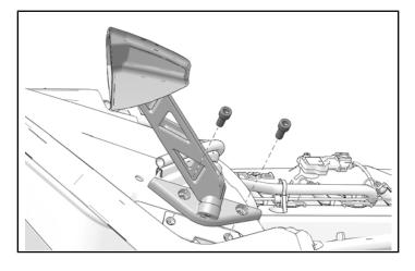
2. Torque mounting screws to specification.
