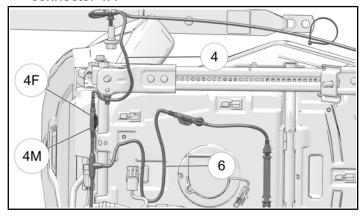
10. Connect right rear interglow harness extension ① connector 4M to rear interglow harness ④ connector 4F.
