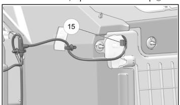
9. Connect left rear interglow harness extension 6 connector 4M to rear interglow light harness 4 connector 4F.
