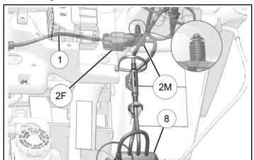
2. Put multicolor interior LED harness ① under ECM mounting bracket. Put routing clip ⑫ in existing hole. Put harness through firewall along existing wiring. Connect 10F plug to rocker switch ⑩. Attach with cable ties ⑪.
