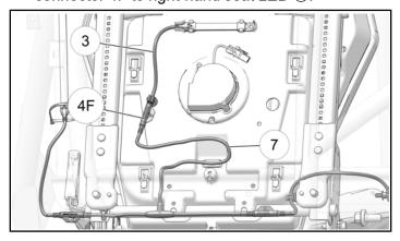
7. Connect right rear interglow harness extension ① to bottom of seat using edge clips ⑤ and ⑥.
