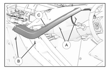
2. Torque two screws to specification.
