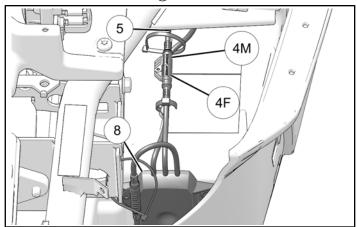
2. Put footwell interior light harness plug through firewall along existing wires. Connect harness 3 4F to footwell LED 2 4M. Attach with cable tie 1.
