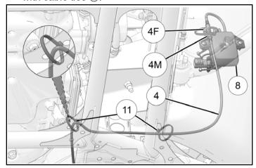
2. Install wire harness ④ along frame rail as shown. Make sure wiring harness is routed above frame components. Attach with cable ties ⑪ and edge clips ⑤.
