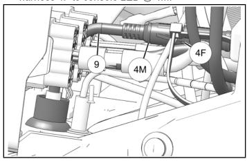
6. Put footwell interior light harness (5) through firewall following existing wiring. Connect footwell interior light harness ⑤ plug 4F to footwell LED ② plug 4M. Attach with cable ties 11.
