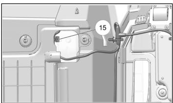
6. Connect right rear interglow harness extension ① connector 4F to right-hand seat LED ③.
