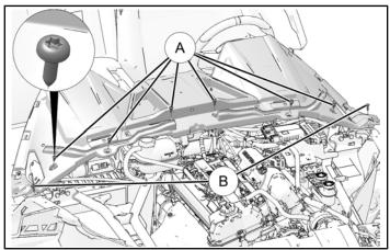
3. Torque eight screws to specification.
