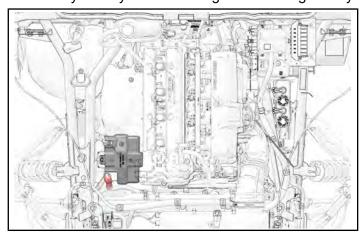
2. Remove negative (–) battery terminal bolt and disconnect negative (–) battery cable.
