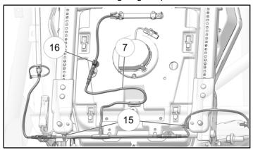
8. Insert long lead from T connector of right rear interglow harness ④ into cabin through opening in bottom of vehicle, clip to seat base with clip ⑤.
