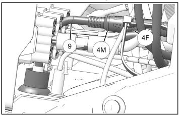
6. Put footwell interior light harness ⑤ through firewall following existing wiring. Connect footwell interior light harness ⑤ plug 4F to footwell LED ② plug 4M. Attach with cable ties ⑪.
