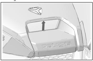
4. Pull hood upward and forward, rotating hood to a vertical position.
