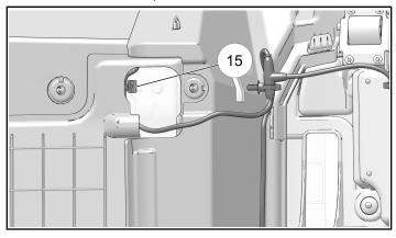
6. Connect right rear interglow harness extension ⑦ connector 4F to right-hand seat LED ③ . Clip to vehicle using ⑤.
