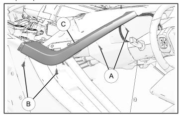
2. Torque two screws to specification.
