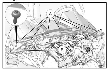
3. Torque eight screws to specification.
