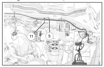
5. Put console LED wiring through firewall along existing wiring. Connect footwell interior light harness 4F to console LED (9) 4M.
