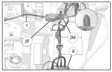
2. Put multicolor interior LED harness ① under ECM mounting bracket. Put routing clip ② in existing hole. Put harness through firewall along existing wiring. Connect 10F plug to rocker switch ⑩. Attach with cable ties ⑪.
