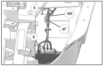
2. Put footwell interior light harness plug through firewall along existing wires. Connect harness (§) 4F to footwell LED (2) 4M. Attach with cable tie (f).
