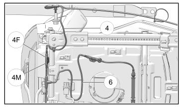
10. Connect right rear interglow harness extension ① connector 4M to rear interglow harness ④ connector 4F.
