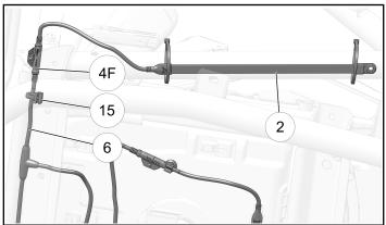
5. Insert left rear interglow harness extension into cabin through opening in bottom of vehicle, clip to seat base with clip (5).
