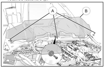
2. Torque fasteners to specification (if applicable).
