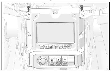
4. Press tabs on back of switch panel to remove switch bezel. Remove switch retainer.
