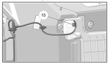
9. Connect left rear interglow harness extension 6 connector 4M to rear interglow light harness 4 connector 4F.
