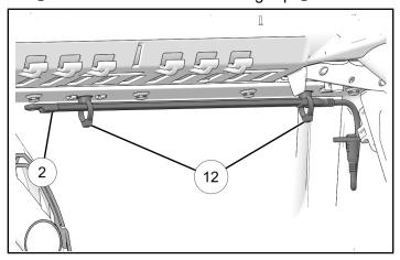
3. Put edge clips ③ in opening above steering column so LED mounts above visor closeout. Put LED strip ② with lights facing down and attach using edge clips ③.
