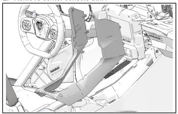
3. Remove and keep two display center fasteners. Move display center away from mounting position and disconnect wiring. Remove display center.
