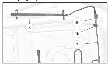
8. Insert right rear interglow harness extension into cabin through opening in bottom of vehicle, clip to seat base with clip (5).
