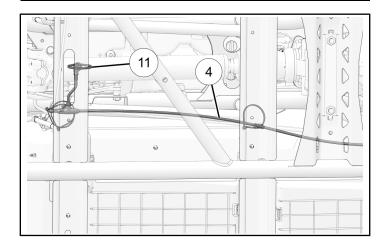
3. Connect left rear interglow harness extension ① connector 4F to left seat LED ③. Clip harness ① to edge clip ⑤.
