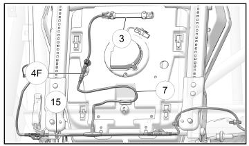
7. Connect right rear interglow harness extension ① 4F to right-hand rocker LED ②. Clip to vehicle using edge clip ⑤.
