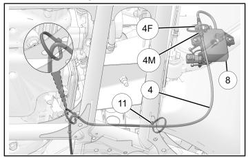
2. Install wire harness ④ along frame rail as shown. Make sure wiring harness is routed above frame components. Attach with cable ties ⑪.
