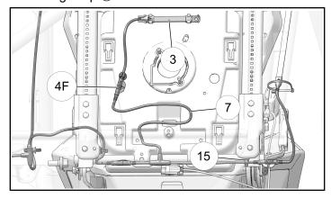
4. Connect left rear interglow harness extension **6** 4F to left-hand rocker LED **2**. Clip to edge clip **5**.
