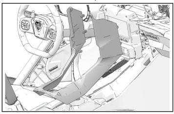
4. Install two retained push pins from center console trim.
