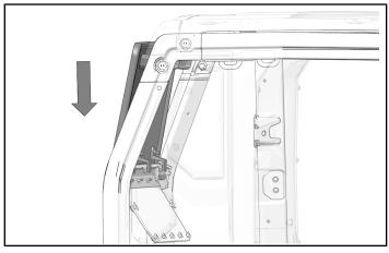
2. Tilt the top of the window into the window frame.
