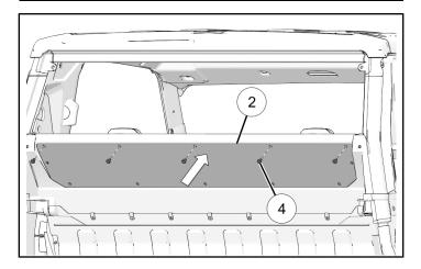
3. Install seven push-pin rivets (4) at sides and bottom of poly window.
