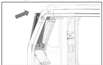
3. Turn the handles upward to lock the window into place.
