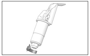
4. Engage Lock & Ride® clamp to secure cooler.
