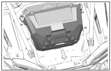
2. Install two Lock & Ride<sup>®</sup> anchors<sup>3</sup>. Make sure mounting holes in vehicle and cooler are aligned.
