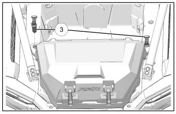
3. Lock & Ride<sup>®</sup> assemblies may need adjustment. Tighten or loosen bottom nut depending on fitment.
