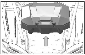
3. Install two Lock & Ride® assemblies ® in two aligned mounting holes.
