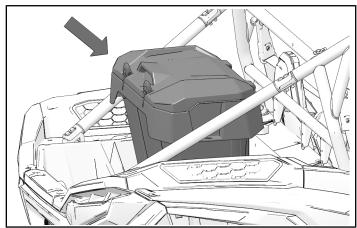
2. Move front of storage box to align Lock & Ride® holes in storage box with those in cargo box.
