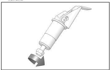
5. Make sure Lock & Ride® assemblies are fully seated before closing top lever and securing storage box.
