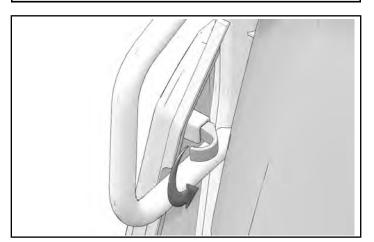
3. Install upper rocker panel with four retained pushpin rivets.
