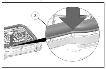
3. Install the seat base seals ② onto the bottom of the front seat (multi-passenger vehicles only).
