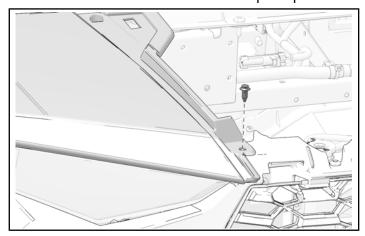
3. Attach rear of outer hood with one retained screw. Torque outer hood screws to specification.
