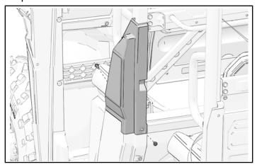
3. Loosen, but do not remove, screw on retaining hook. Rotate hook until it is free of bolster tube.
