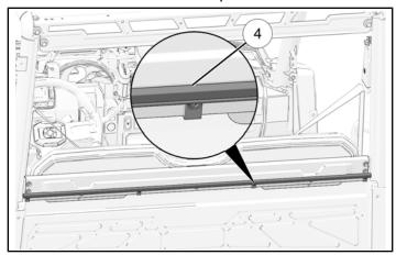
5. Identify the installation location on the LH side of vehicle for C-pillar seal (s). Clean installation surface as required.
