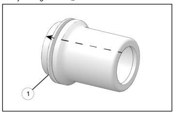
2. Identify the installation location on the brake cylinder for the brake cylinder grommet ①. Clean installation surface as required.
