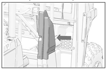
2. Rotate hook over bolster tube.
