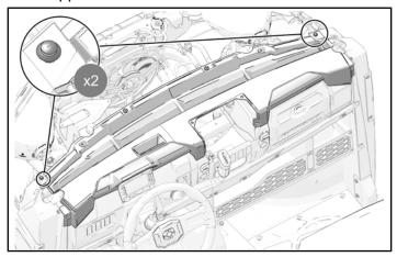
3. Install four retained push-pin rivets into rear face of upper dashboard.
