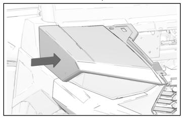
2. Attach front of outer hood with one push-pin rivet.
