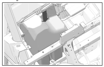
2. Install glove box with three retained push-pin rivets.
