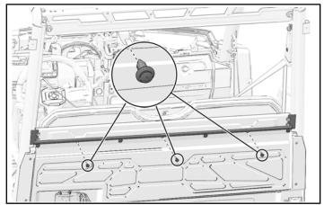
11. Identify the installation location on the LH side of vehicle for LH rubber grommet (1). Clean installation surface as required. Install grommet through the LH side of the rear close off panel.
