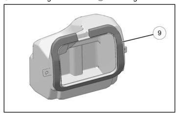
4. Peel the adhesive backing from the foam, then insert the foam onto the front of the glove box.
