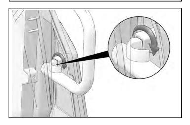
3. Install bottom of ROPS pillar cover with two retained push-pin rivets.
