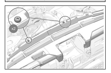
2. Install two retained push-pin rivets into front edge of upper dashboard.
