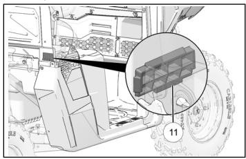
13. Remove and keep one push-pin rivet from the RH lower rocker panel.
