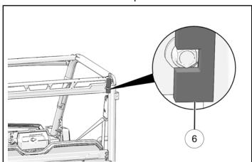
4. Peel the adhesive backing from the foam, then insert the foam onto the rear upper cab frame plate.
