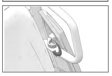
3. Install upper rocker panel with four retained pushpin rivets.
