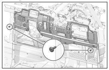
4. Remove and keep the six push-pin rivets from the lower dash panel.
