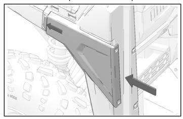
2. Install side access panel with four retained pushpin rivets.
