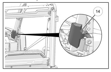
4. Peel the adhesive backing from the seal, then insert the seal onto the right front cab frame tube.
