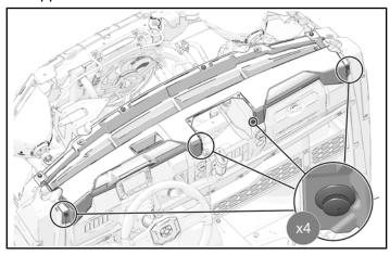
4. Torque two upper dashboard screws to specification.
