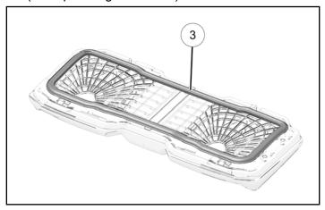
2. Carefully press the edging of the seat base seal ③ into the molded lip on the bottom of the seat.
