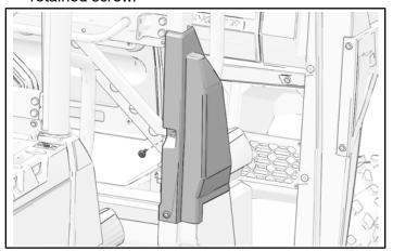
5. Tighten screw in retaining hook until it is fully seated.
