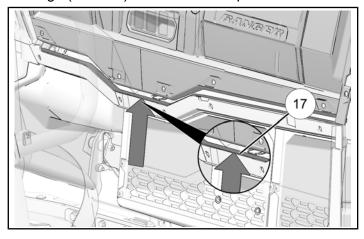
6. Lift the bottom of the lower dash panel upwards and install the bottom dash foam <sup>®</sup> onto the top edge (LH side) of the front floor panel.
