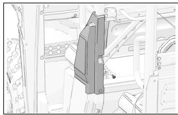
2. Remove and keep two push-pin rivets from ROPS pillar cover.
