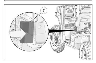
18. Install the one push-pin rivet back into the LH lower rocker panel.
