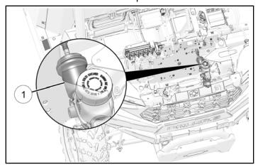
3. With the slit side facing downward, slide the grommet over the top of the brake cylinder shaft.
