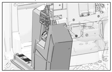
17. Pull back the lower rocker panel to gain access, and insert the rocker foam ① between the rear close off panel and the seat frame.
