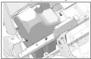
2. Open glove box and remove one screw from inside.
