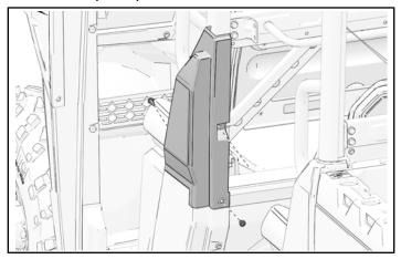
4. Install middle of ROPS pillar cover with one retained screw.
