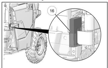
2. Identify the installation location on the LH side of vehicle for the door hinge foam (6). Clean installation surface as required. Slide the foam over the door hinge bracket.
