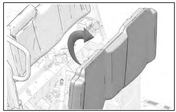
2. Lift seat up and remove from lower hinge brackets.
