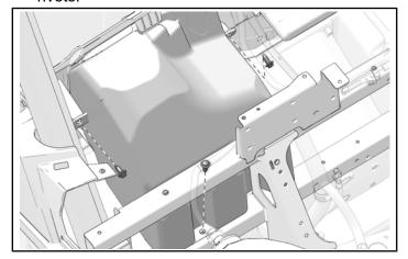
3. Open glove box and install one screw. Tighten until fully seated.
