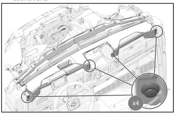
2. Remove and keep two push-pin rivets from upper dashboard.
