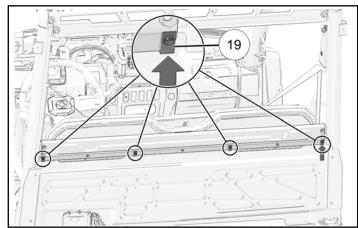
4. Peel the adhesive backing from the rear close out cab frame seal ④, then insert the seal onto the back of the mid cab frame plate above the holes.
