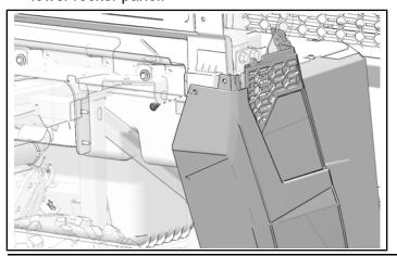
14. Pull back the lower rocker panel to gain access, and insert the rocker foam ① between the rear close off panel and the seat frame.
