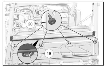
10. Install the three retained push-pin rivets into the back of the rear close off panel.
