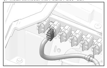
6. Route horn harness towards driver's side. Put harness into clips at taped locations.
