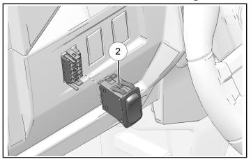
10. Put horn switch ② into opening and push until it snaps into place.
