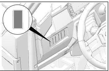
8. Put switch connector through cut hole.
