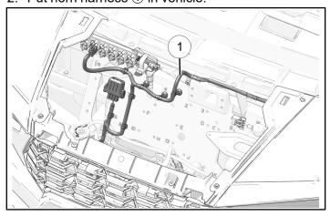
3. Attach fuse relay box and harness push-darts into panel, as shown.
