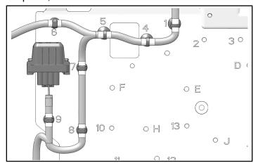
4. Route two horn connectors down towards horn and install into back of horn assembly. Attach excess harness to chassis with edge-clips.
