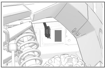
9. Install switch connector to horn switch ②.
