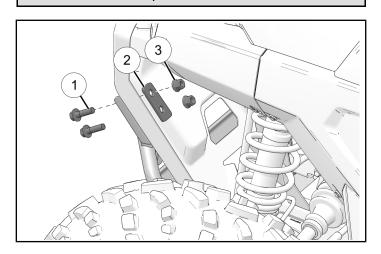
4. Install bottom of plow mount with one carriage bolt6 and one nut5. Torque two nuts to specification.
