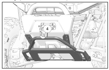
3. Put two screws ① through plow mount and bumper. Loosely install with mounting plate ② and two nuts ③ on the other side.
